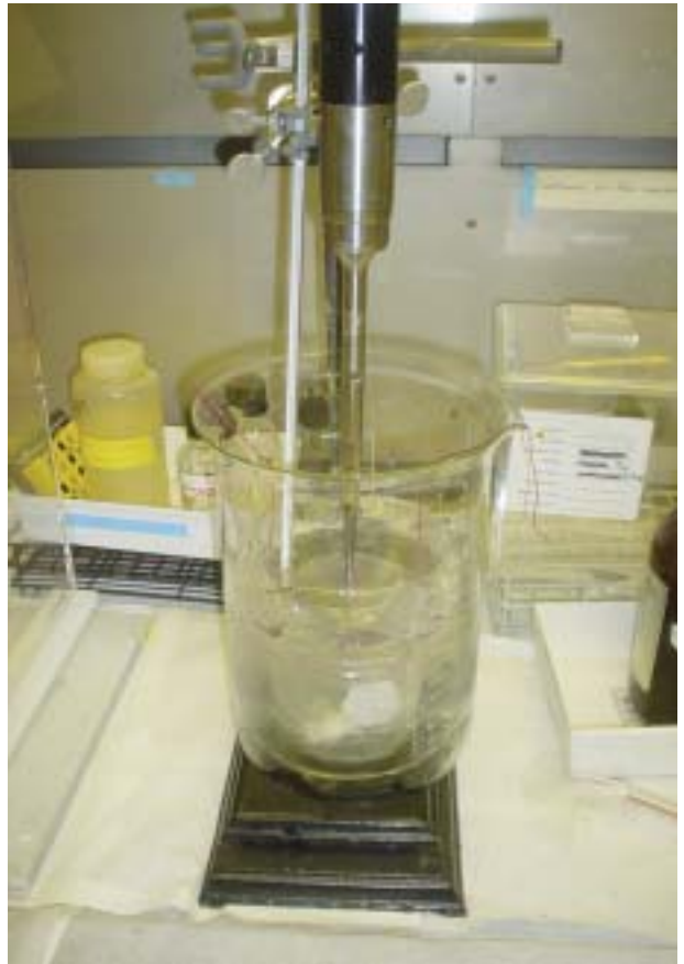
This laboratory apparatus was used to develop a process in which NanoMatrix's high-velocity liquid jets helped adhere a family of next-generation coatings to materials that would otherwise not adhere very well.
