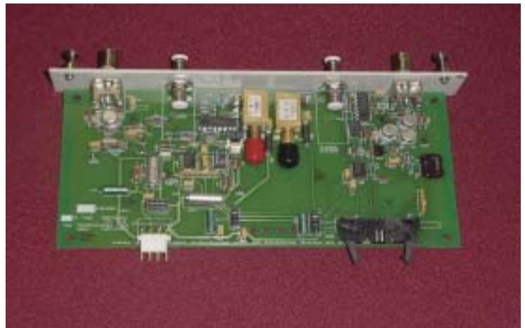
Omni Technologies' FOTR-125 is a redundant fiber-optic transceiver that remotely transfers high-speed digital data.
