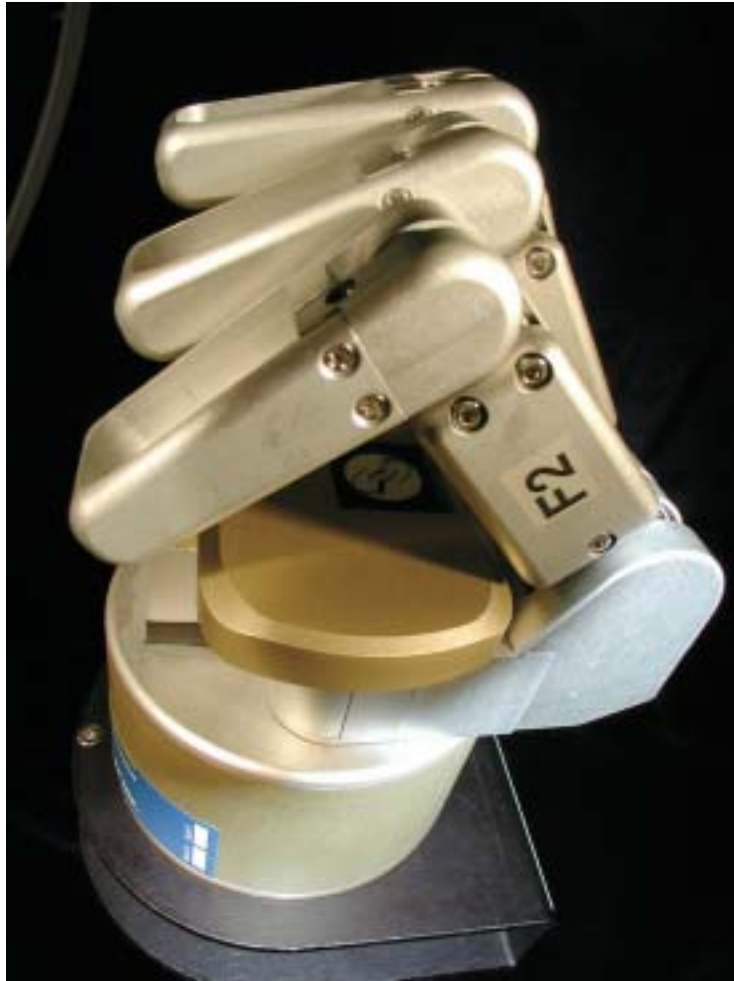
The BarrettHand,™ a multi-fingered programmable grasper, can pick up objects of various shapes and sizes.
