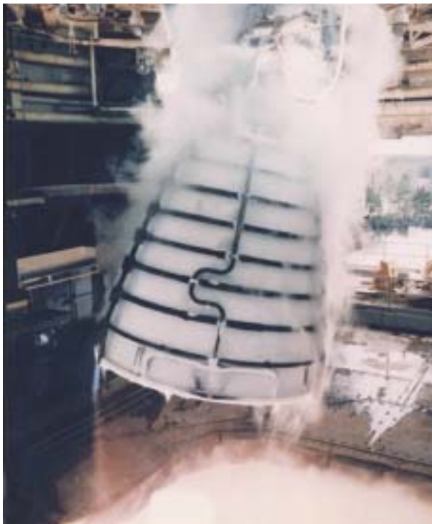
A close-up view of a Space Shuttle Main Engine during a test at Stennis Space Center shows how the engine is rotated to evaluate the performance of its components under simulated flight conditions.
