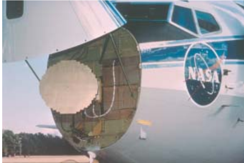
Langley Research Center's Boeing 737 research aircraft is fitted with a Doppler radar wind shear detection system that sends a beam well ahead of the airplane to detect microbursts.
