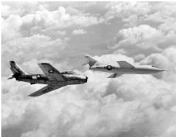
This mid-1950s photograph shows the Douglas D-558-2 and the North American F-86 Sabre chase aircraft in flight. Both aircraft display early examples of swept wing airfoils.
