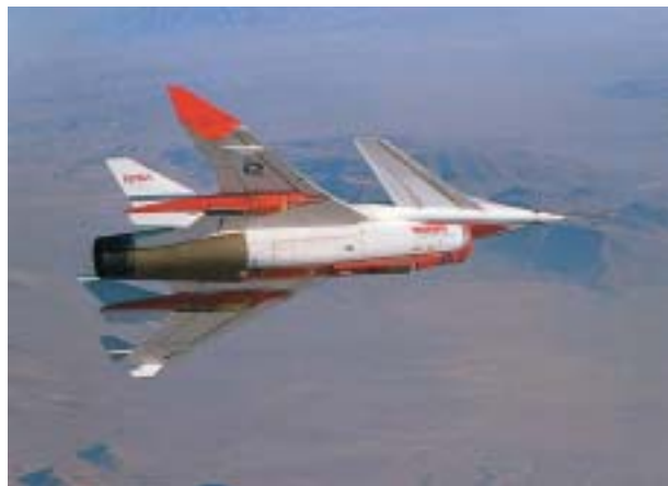
The Highly Maneuverable Aircraft Technology subscale research vehicle, seen here during a research flight, was flown by Dryden Flight Research Center from 1979 to 1983. The aircraft demonstrated advanced fighter technologies that have been used in the development of many modern high performance military aircraft.
