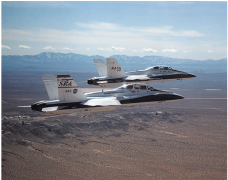
Two F/A-18B aircraft fly in tight formation using the autonomous flight functions developed at Dryden.
