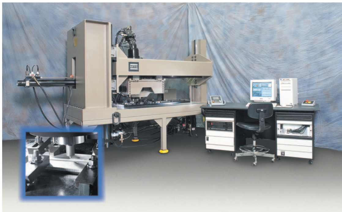
The MTS Friction Stir Welding Process Development System uses the NASA-developed self-adjusting, retractable pin tool to offer welding capabilities that were previously unachievable with other welding systems.
