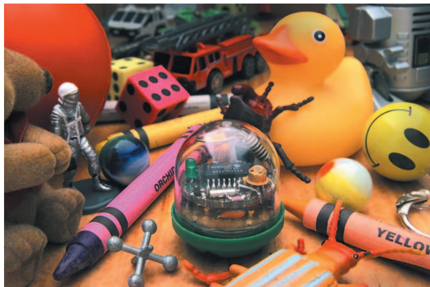
This small device, called a pod, can be collected in groups together to form a new type of instrument called a Sensor Web. Each pod contains sensors that collect information from the surrounding environment and communication chips that transmit the data to other pods. Hopping from pod to pod, the data eventually arrives at a primary uplink where it can then be sent to an orbiting satellite for transmission back to Earth.
