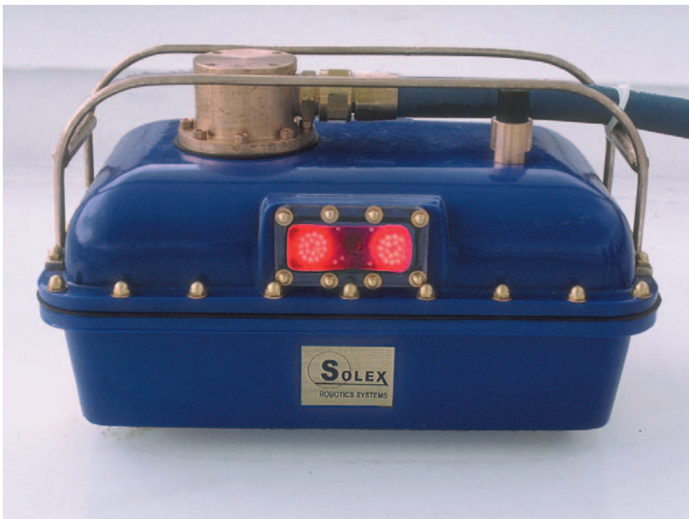
The submersible Maverick robot allows for the safe inspection and cleaning of storage tanks.
