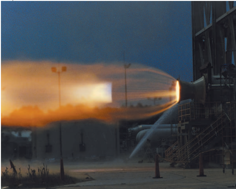
A TRW 650K Low Cost Pintle Engine undergoes hot fire testing at Stennis' E-1 test stand. The test article achieves a high level of power without a high cost because of the simplicity of its design. Physically, the TRW 650K is the second largest engine ever tested in the United States.
