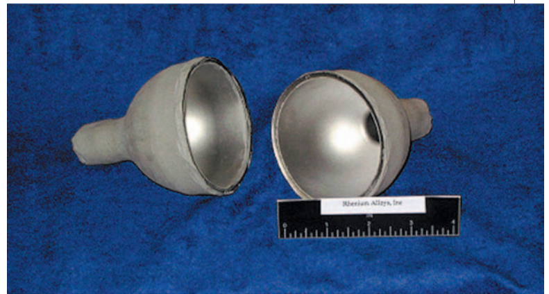
Rhenium Alloys, Inc., uses NASA-developed methods to manufacture custom parts from rhenium, such as the two domes displayed here.
