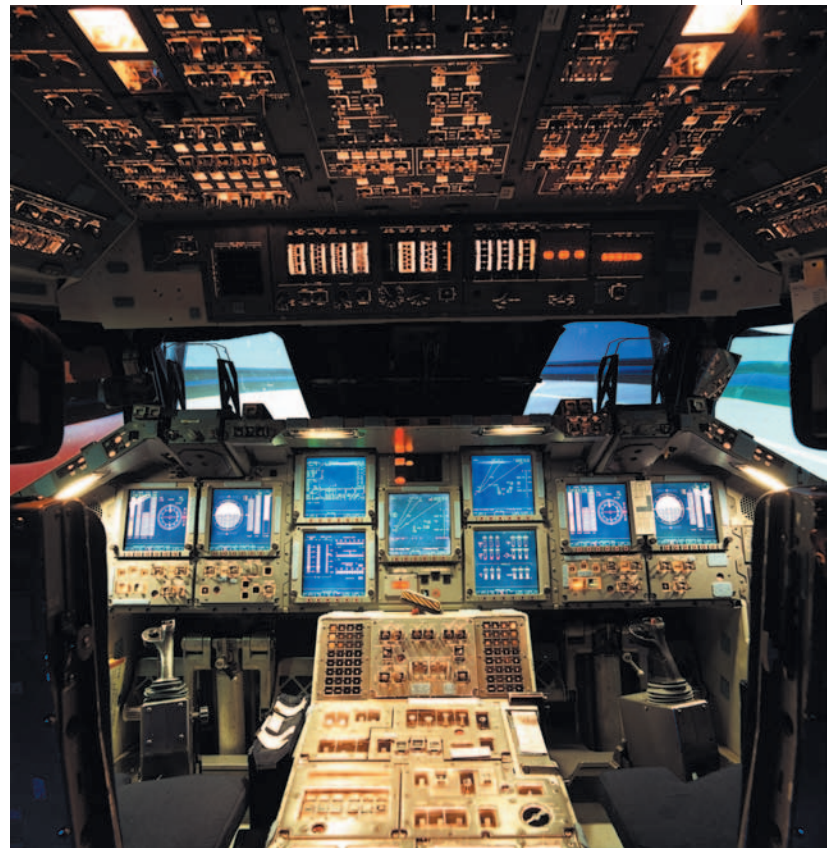
The Multifunction Electronic Display Subsystem (MEDS), otherwise known as the “glass cockpit,” is shown in the fixed base Space Shuttle mission simulator at Johnson Space Center’s Mission Simulation and Training Facility. MEDS is installed on the Space Shuttle Atlantis.
