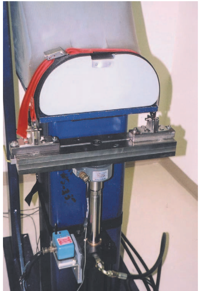
Engineers from NASA's Johnson Space Center helped Aircraft Belts, Inc. to develop a hydraulic test system that provides detailed data about the load placed on aircraft restraints.
