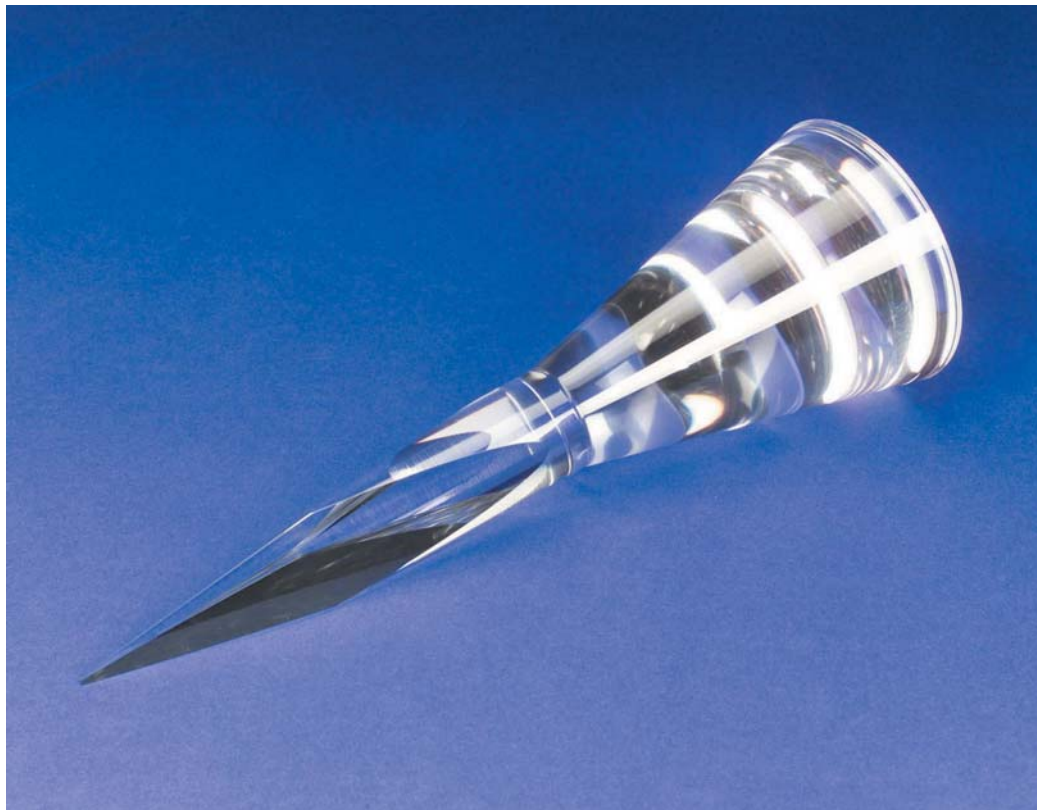
Glenn Research Center's sapphire refractive secondary concentrator will be used with primary collector-concentrators to focus solar energy. The solar energy can be used in power conversion systems, thermal propulsion systems, and solar furnaces.
