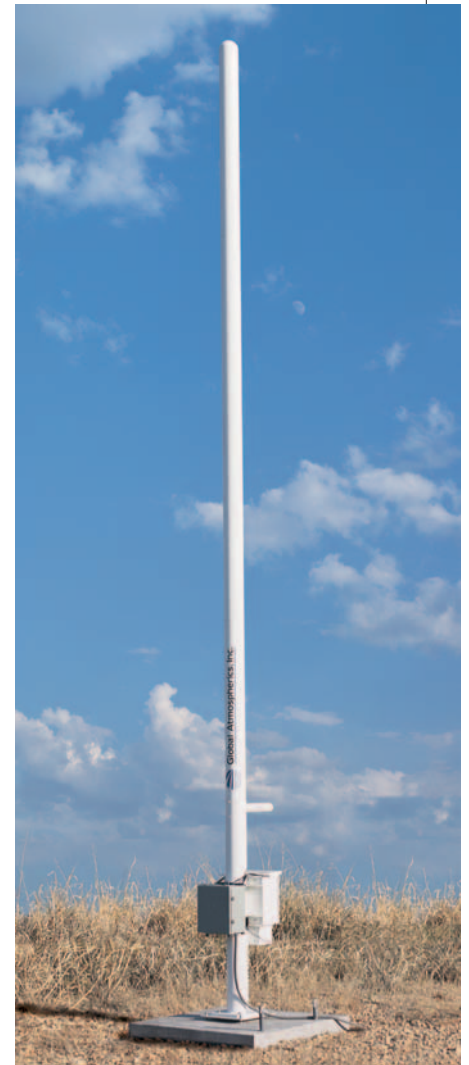
The LDAR II fiberglass lightning mast contains signal processors that provide data to a computer where the user can then interpret the extent of lightning hazard.
