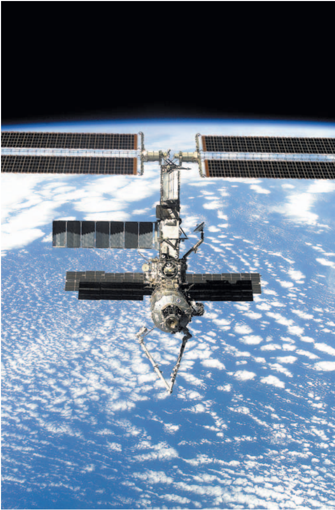
Backdropped against the blue and white Earth and sporting a readily visible new addition in the form of the Canadarm2 or Space Station robotic arm, the International Space Station was photographed following separation from the Space Shuttle Endeavour.
