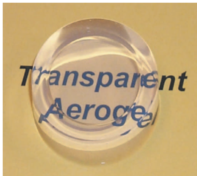
Aerogel is the lightest solid known to man and is sometimes referred to as "solid smoke" or "frozen smoke."
