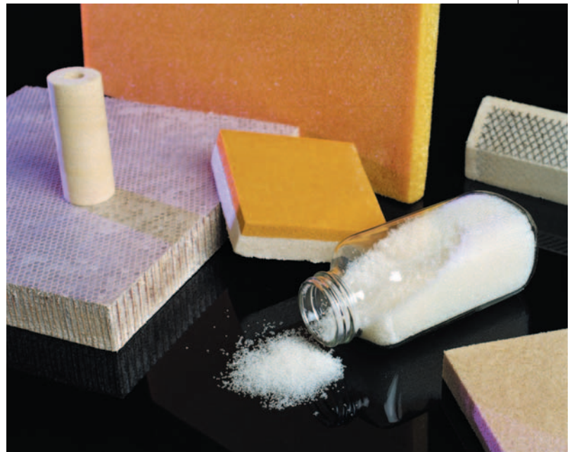
SORDAL, Inc. offers NASA's TEEK polyimide foam in several forms, including microspheres, preprocessed neat and syntactic foam, and foam-filled honeycomb.
