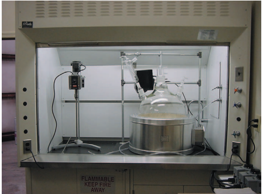
Unitech's custom lab reactor can generate multiple sample requests of RP46 as well as small production quantities of up to two tons per month.
