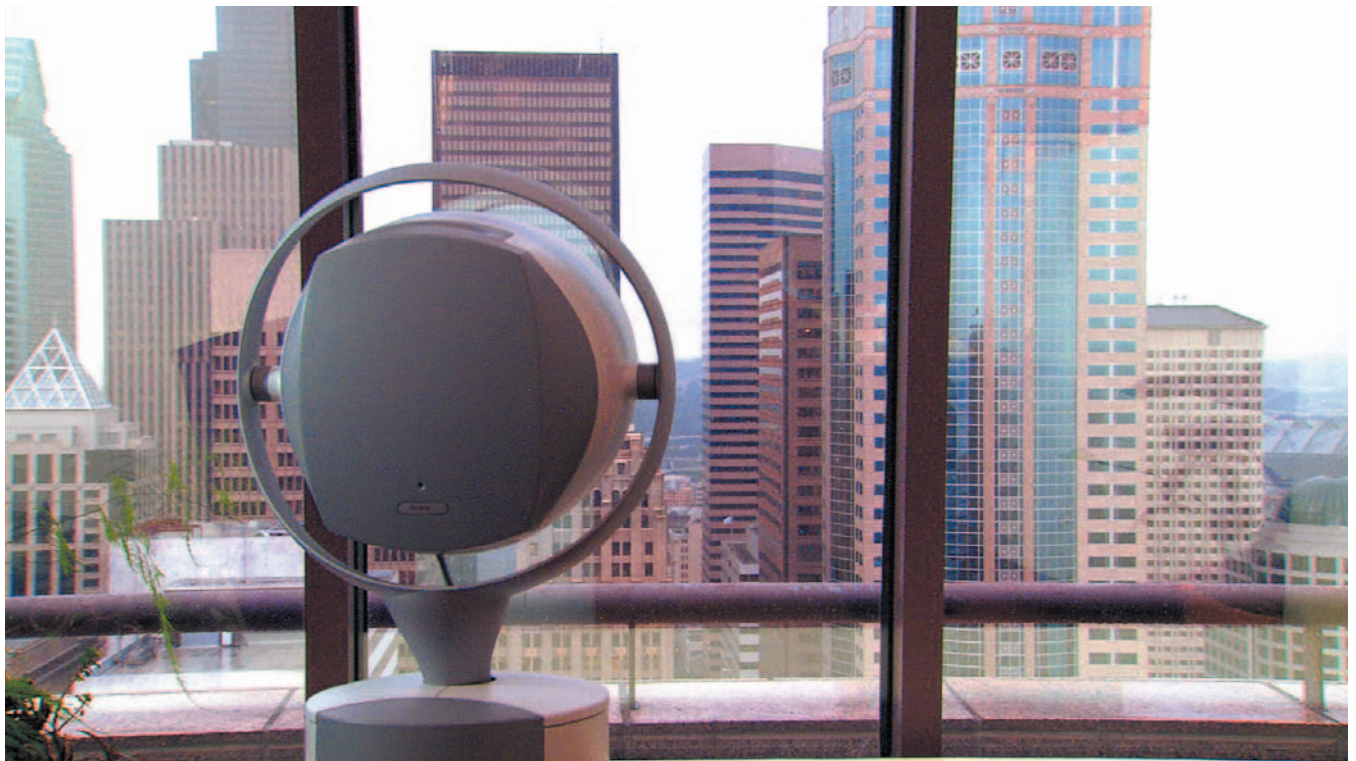
Terabeam's Fiberless Optical™ Network transmits broadband data from office buildings to the nation's wide-area networks (WANs) through the air.
