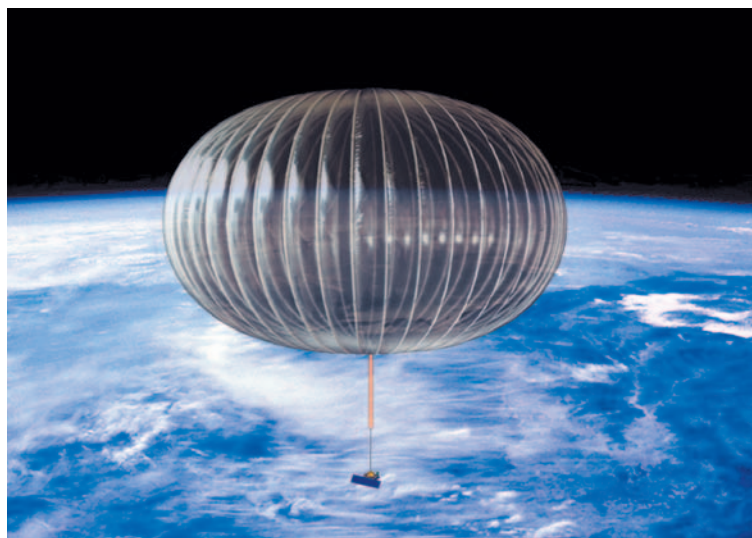
An artist's concept of NASA's Ultra Long Duration Balloon (ULDB), a revolutionary new balloon capable of supporting scientific observations above 99 percent of the Earth's atmosphere for durations approaching 100 days.
