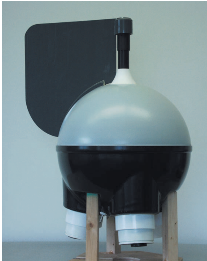
ADOS is used for the in situ measuring of ocean surface layer properties such as surface winds, surface thermal structure, and ocean color. The information gathered by ADOS is then collected via satellite.
