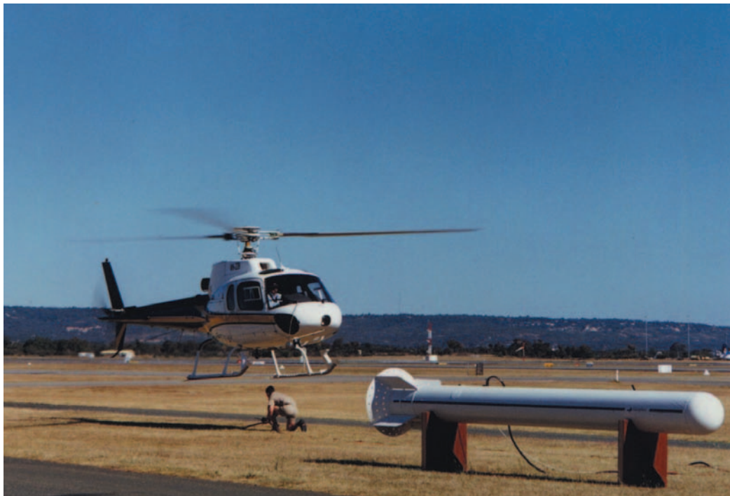
The GEM-2A airborne sensor is commercially used for surveying large areas of land, in search of minerals, metals, and hydrocarbons.
