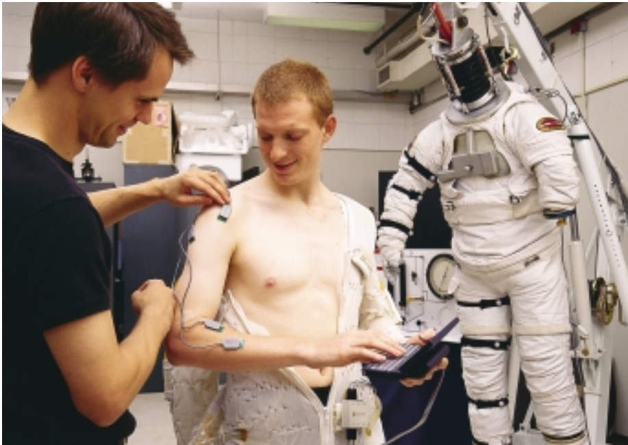
The MyoMonitor® is being evaluated to study the muscles of astronauts in the weightless environment of space.
