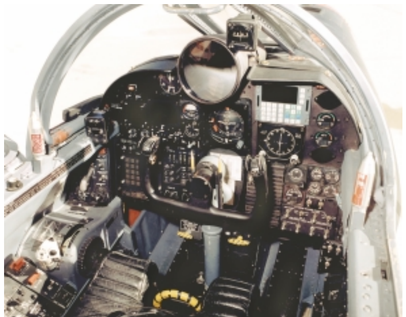
The cockpit of the ER-2, one of the planes used in NASA's Airborne Science Program.
