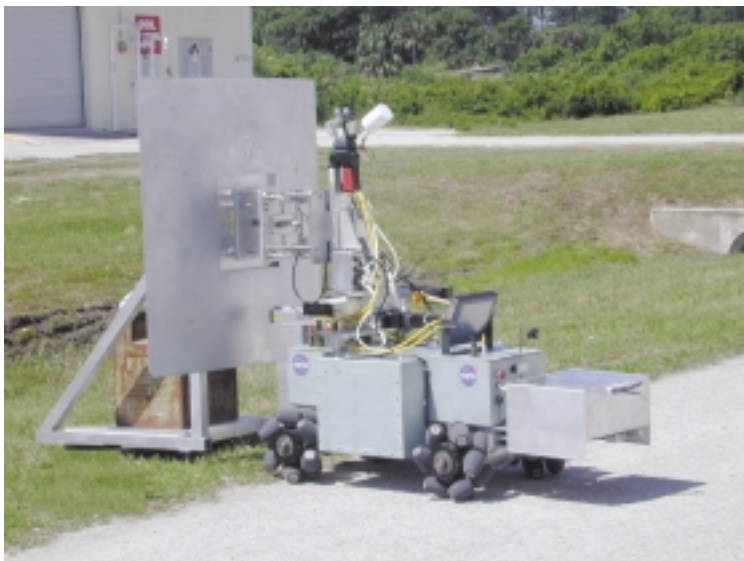
The OmniBot Mobile Base can be used in hazardous environments to perform remote inspections, site surveys, and operations.
