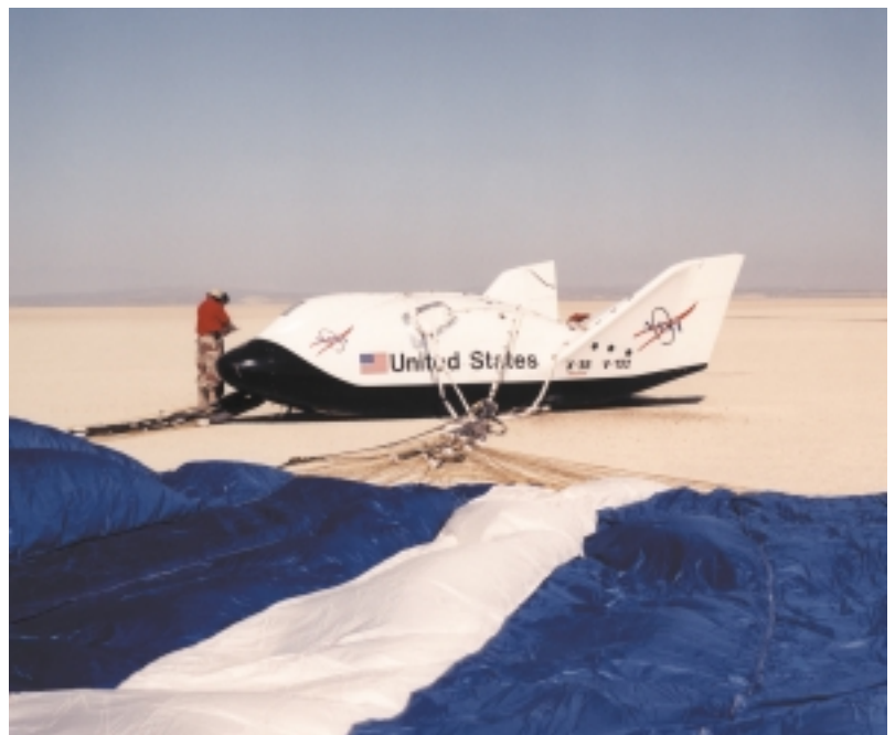
The X-38 with its parachute deployed after a successful flight test in the California desert.
