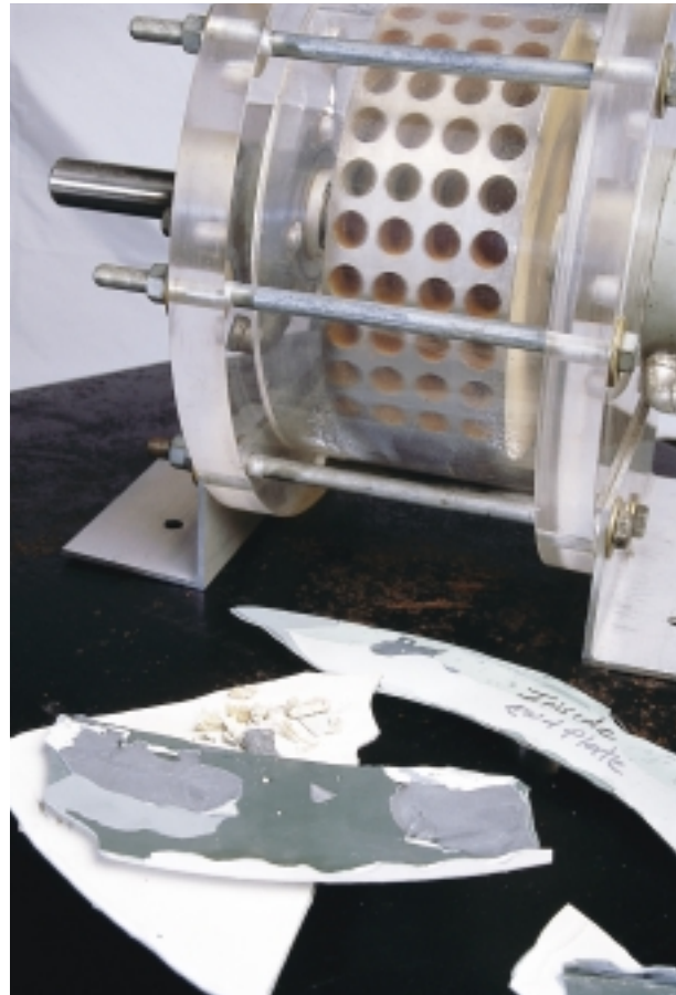
NASA engineers solved a design problem with Hydro Dynamics' rotor for use in the Hydrosonic Pump.™ The holes in the rotor produce microscopic bubbles, preventing the buildup of impurities (scale).
