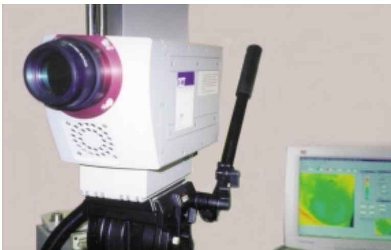
OmniCorder Technologies, Inc.'s BioScan System TM detects blood flow differences associated with cancerous cells.
