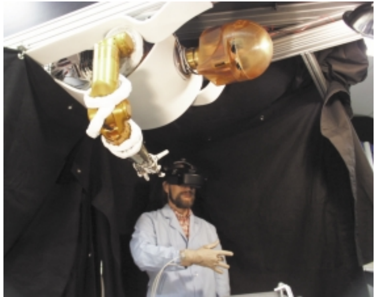
A Johnson scientist manipulates the Robonaut system, which includes a mechanical hand capable of moving with dexterity similar to a human.
