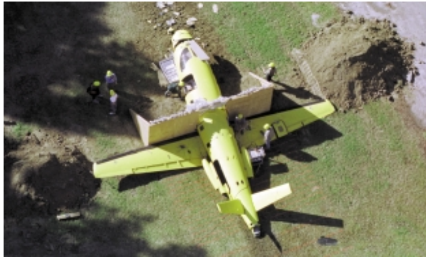
Langley researchers perform various crash tests on airplanes, such as the one shown here, in an effort to improve aircraft safety performance.
