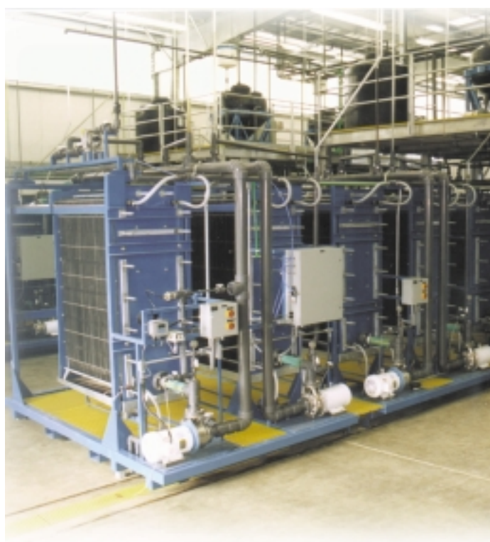
Osmotek, Inc.'s Direct Osmosis treatment system is being used to keep a landfill's surroundings clean.
