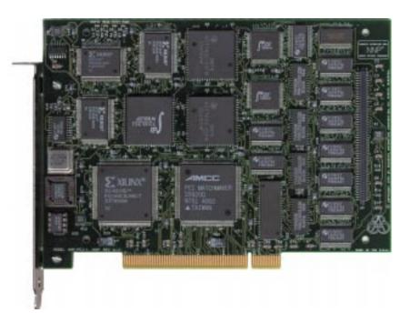
Accurate Automation Corporation's neural processor, the NNP®, was developed using the interconnectedness of the human brain as a model. of Chattanooga, Tennessee, developed the only Multiple-Instruction/Multiple-Data (MIMD) neural network processor on the market. The product is called the NNP<sup>®</sup> and is utilized in a number of computational applications.
