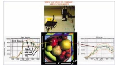
OptoKnowledge Systems, Inc.'s hyperspectral imaging system can be used in applications such as food inspection.
