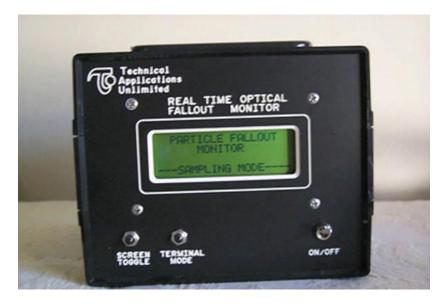
Technical Applications Unlimited, Inc.'s Real-Time Optical Fallout Monitor is designed for use in many areas of industry. accumulation of potentially damaging dust and fibers on delicate payload components.
