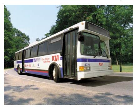
traffic, the Hybrid Electric Transit Bus continues to run at near peak efficiency while stopped. The power is stored and used when the bus needs a boost, such as when climbing steep hills.
