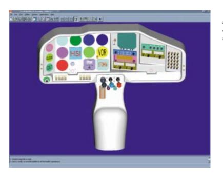
The company started work on its instrument panel concept by creating a 3-D computer model.
