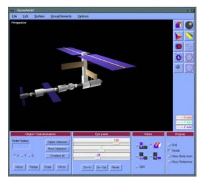
Dynacs Engineering Company, Inc.'s Dycom is a multibody dynamics and control system simulation tool. proved highly accurate when ground simulations were contrasted with both original manufacturer data and actual data taken during Shuttle missions.
