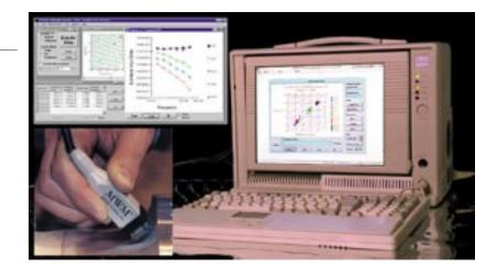
tested the system for performing very early stage crack detection in stainless steel, aluminum, and other materials.
