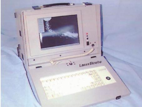
Control Vision, Inc.'s LaserStrobe<sup>®</sup> and PyroCam<sup>®</sup> systems can yield high-resolution video images of high-energy industrial processes. blind to the radiation coming from the process. The rapid-fire laser pulse also freezes powder particles in flight.
