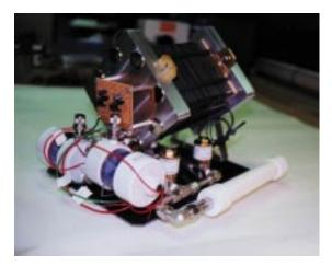
ElectroChem's EC-PowerPak200 churns out 200 watts of power. Versatile fuel cells offer high energy while being virtually pollution free.
