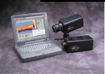
Stress Photonics, Inc.'s GFP 1000 acquires full-field images quickly and efficiently, detecting cracks in structures.
