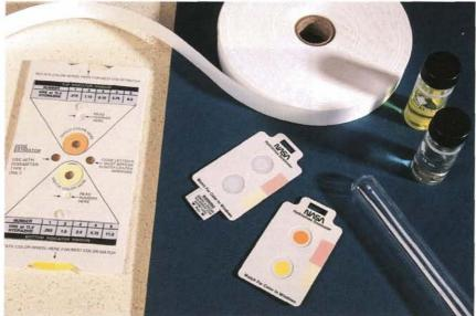
GMD Systems' Hydrazine Badge changes color when its wearer is exposed to a chemical containing a hydrazine component.
