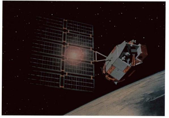
Clark's sister satellite— Lewis—has an advanced remote sensing imager that significantly broadens the range of Earth features that can be analyzed. Both satellites will operate as commercial remote sensing systems in addition to their NASA assignments as technology demonstrators.
