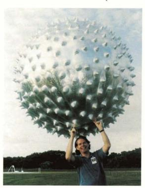
The Jimsphere wind measurement balloon is made of lightweight radar-reflective materials. such inflatable, known as the "Jimsphere," is of particular interest because, although developed more than 30 years ago, it remains the standard at all U.S. missile/ launch vehicle ranges for obtaining accurate upper level wind data.
