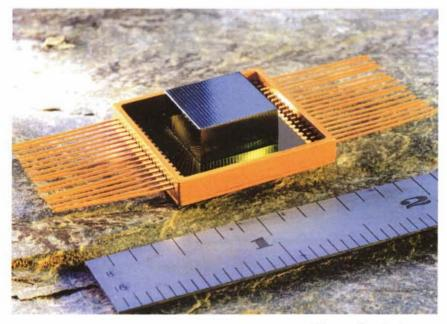
A Memory Short Stack is a cube-shaped package of integrated circuits.
