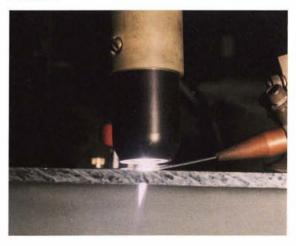
A small version of the B&B torch is used in commercial sheet metal welding.
