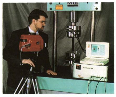
The DeltaTherm 1000 stress measurement system combines digital signal processing technology with an infrared camera.
