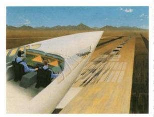
Future jetliners may employ a design technique that eliminates forward-facing cockpit windows and substitutes a 3D computergenerated color display to give the pilots "synthetic vision" on takeoffs and landings. Already flight tested, this system could save thousands of pounds of weight that could be more productively used. weather, reducing terminal delays and cutting costs for airlines and passengers.
