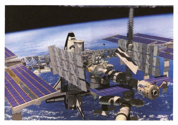
This concept views the station from the opposite (aft port) end. In the foreground (lower right) is the Russian Service Module, with living and working room for three crew members. Next, toward center of photo, is the FGB energy block, then (near the Orbiter) the U.S. lab module. The vertically-mounted cylinder below it is the U.S. habitation module.
