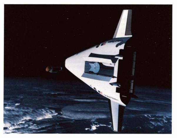
In development for first flight in 1999 is the NASA/Lockheed Martin X-33 Advanced Technology Demonstrator, intended as the prototype of a 21st century low-cost-to-orbit reusable launch vehicle. days, not months, to turn around; dozens, not thousands, of people to operate; with launch costs that are a tenth of what they are now. Our goal is a reusable launch vehicle that will cut the cost of getting a pound of payload to orbit from \$10,000 to \$1,000."
