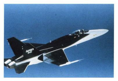
NASA's veteran F-18 HARV research aircraft concluded a decade-long flight test program that explored aircraft maneuverability and controllability at high angles of attack.
