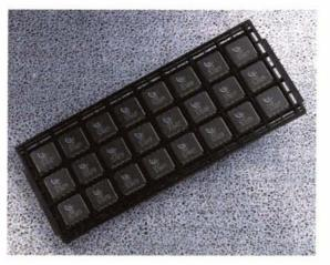
A unique high performance chip, developed by the TelSys group when it was a NASA unit, is produced in units of 24.
