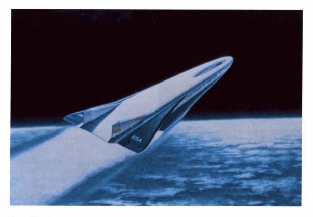
One possible configuration of a future airbreathing hypersonic vehicle that could cruise within the atmosphere at speeds up to Mach 10.
