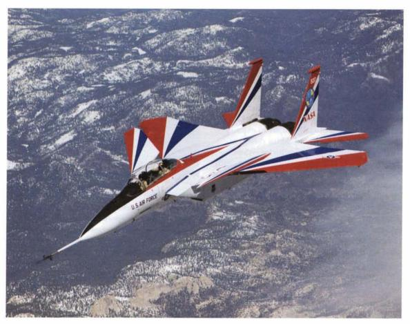
The F-15 ACTIVE is exploring a vectored thrust system that could replace conventional aerodynamic control surfaces. to explore new technologies and new flight regimes. NASA conducts such programs independently or in cooperation with U.S. industry and the Department of Defense, sometimes in cooperation with international development teams.
