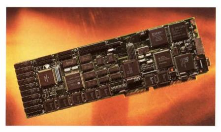
The companion OPTIVideo Decoder decompresses the bit stream to provide high quality digital playback.
