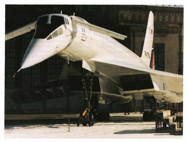
The Russian TU-144LL supersonic flight laboratory employs a mechanical system to "droop" the nose section. This technique is necessitated by the fact that the airplane lands nose high and pilots could not see the runway with the nose in standard flight position. The NASA/industry High Speed Research team is working on an alternative approach (see photo opposite). heavy weight penalty that is not considered acceptable for the second generation vehicle.
