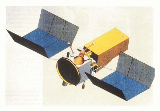
Developed by CTA, Incorporated, the Clark satellite is designed to demonstrate technologies for a new family of satellites featuring reduced cost and compressed development time. ture x-ray detectors, 3D imaging of atmospheric trace gases, and on-board data processing.
