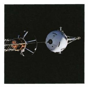
A view of the Tethered Satellite at the start of its deployment from STS-75. The satellite was lost when the tether snapped but the experiment provided considerable useful data.
