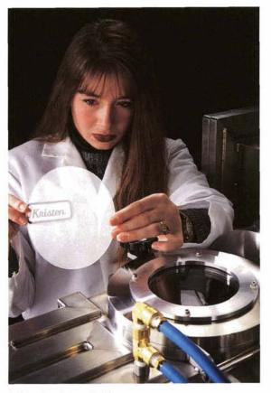
A Barr Associates technician unloads a filter from a chamber where thin film coatings are applied to ultraviolet filters.
