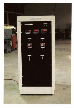
Among the properties of metal hydrides is their ability to store hydrogen in a solid state, an area that has not been widely exploited. Since hydrogen is a common spacecraft propellant, but difficult to store, NASA was interested in the potential of metal hydrides as a means of storing hydrogen in solid state and thus avoiding the hazards of compressed gas or the complexity and boiloff of liquid hydrogen.
