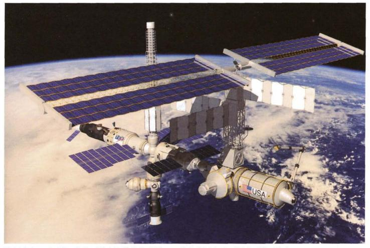
The interim International Space Station will look like this. In the right foreground is the U.S. Laboratory Module and the station's airlock. In the center of the horizontal string of modules is the FGB energy block. The solar power array at top is one of four that will provide power for the complete station. Below the tower is the Russian-built Universal Docking Module and, at bottom, one of two crew transfer vehicles.
