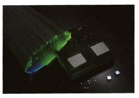
Barr developed an advanced ion-assisted physical vapor deposition process to produce high performance filters for fiber optic communications and other applications.
