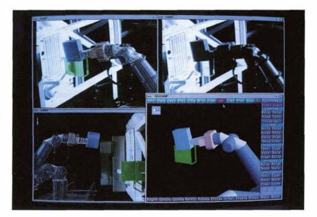
The operator can view the video image of the real world environment (upper right) and the computer's interpretation of the same scene using TELEGRIP.
