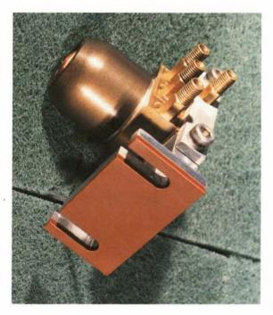
The VPPA concept dates to 1947, but it had never been fully developed; it employs a variable current waveform that enables the welding system to operate for preset time increments in either of two polarity modes for most effective joining of troublesome light alloys such as aluminum and magnesium.
