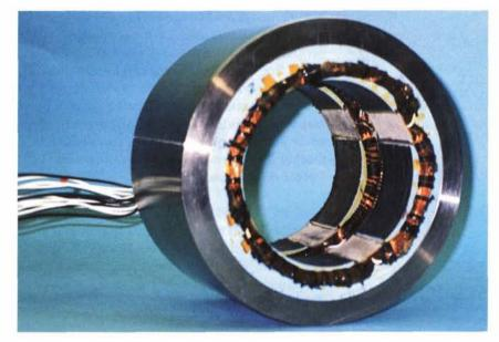
In 1993, Marshall Space Flight Center awarded AVCON a contract to fabricate a set of magnetic bearings, install them in a fixture representing a Space Shuttle Main Engine turbopump, and test them under simulated Shuttle mission conditions. Those tests are under way. The AVCON magnetic bearing permits motion without friction or wear:
