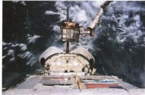
This view of the Orbiter Endeavour's stern shows the Spartan 207 free flyer being recaptured after a day-long research trip away from the Orbiter. It is being jockeyed toward its stowage berth by an astronaut operating the remote manipulator system. the Spartan was grappled and retrieved the following day.
