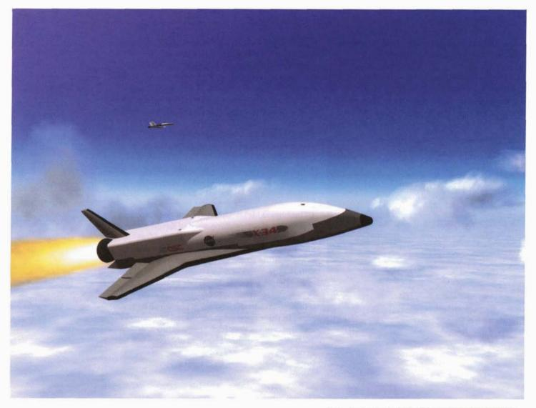
Under development by Orbital Sciences Corporation is the X-34, an experimental vehicle for testing technologies for a single-stageto-orbit launch vehicle. First flight is targeted for 1998.
