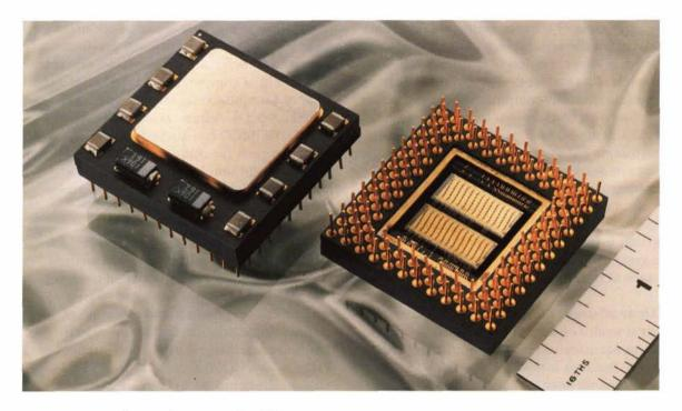
Stack to a spaceborne data recorder. That project significantly advanced the commercialization potential because it called for designing the short stacks so that they would be compatible with such industry standard attachment techniques as wire-bonding and tape-automated bonding; this configuration made Memory Short Stacks usable in virtually all types of electronic assemblies.
