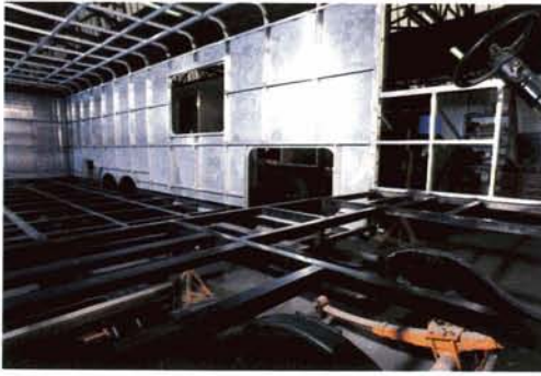
A vehicle frame under construction at Wolverine Western (left). The company's frame technology also originated in NASA software, initially developed to analyze space station configurations.
