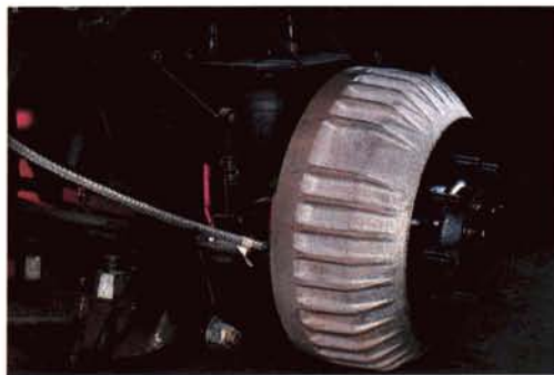
A Wolverine brake drum view from a different angle. The company's chassis employ the spinoff drum brakes on rear axles, disc brakes on the front.
