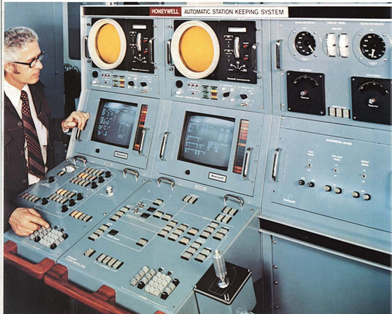
The Honeywell Automatic Station Keeping System, which is based on spacecraft positioning technology, is an anchor-free mooring system for drillships. Using a beacon on the seabed as a reference point, the system computes the ship's location relative to the well and automatically directs fore-and-aft and side-to-side movement to keep the ship properly positioned.
