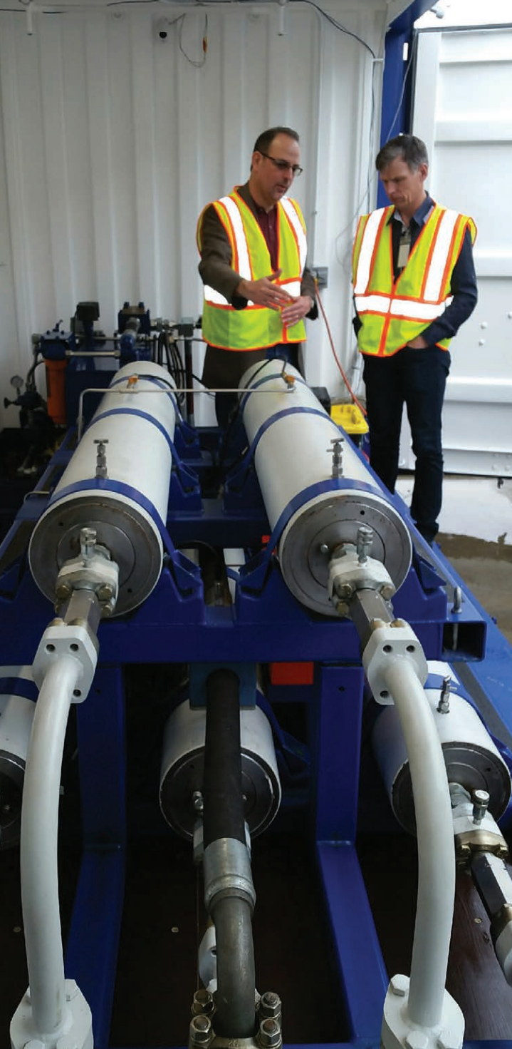
At demonstrations in late 2018 and early 2019, Bastion showed major players in the oil industry how five of its SureShear chambers (left) could power the very blowout preventer that failed to completely sever and seal the drill pipe in the Deepwater Horizon disaster (above). This 15,000-pound SureShear system replaces 170,000 pounds of compressed-gas tanks in a traditional system and severs the pipe about three times as fast.
