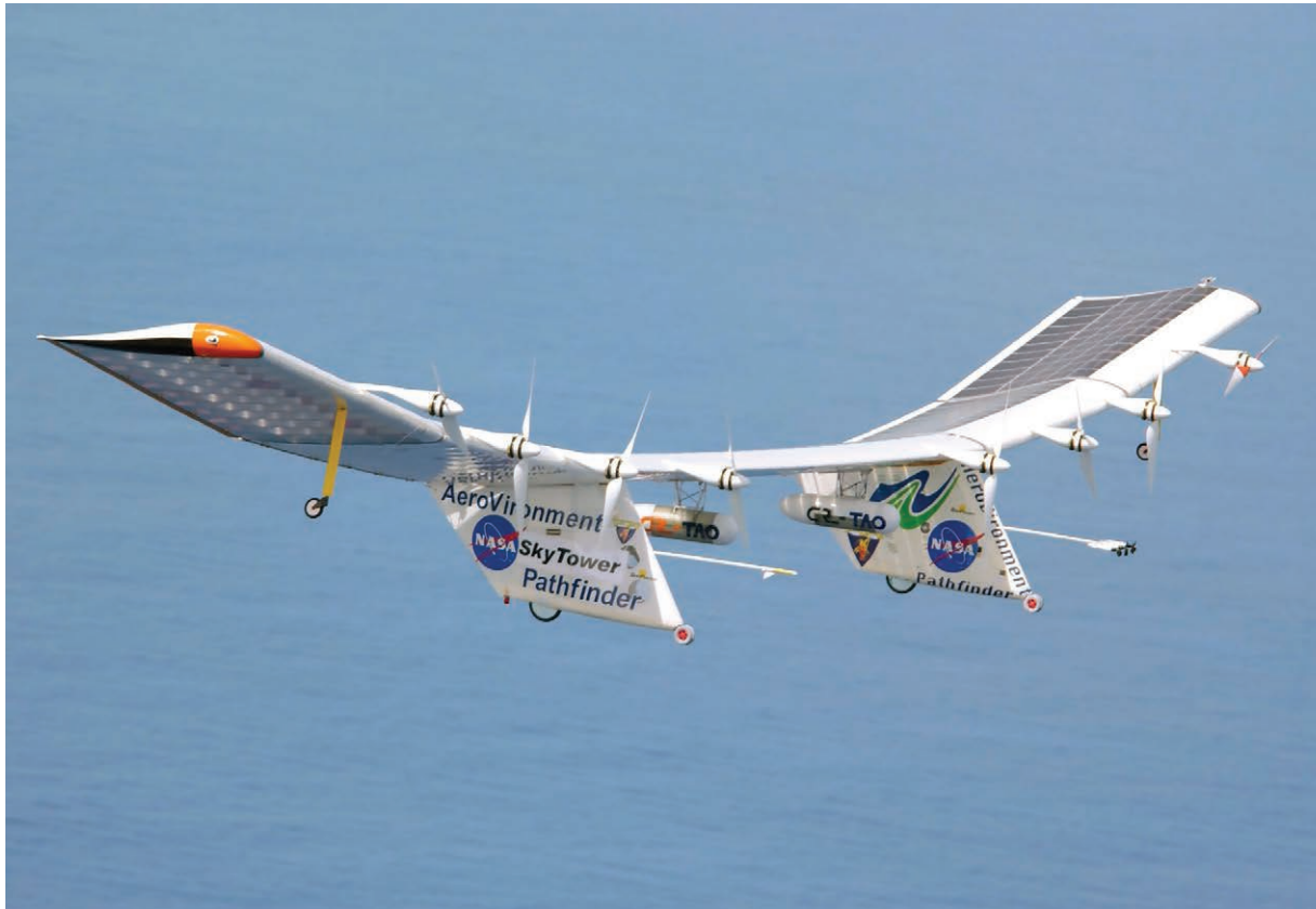
To build the Mars helicopter's rotors, landing gear, and solar panels, the Jet Propulsion Laboratory team turned to a company called AeroVironment, which had built up expertise in thin-atmosphere flight while working with NASA on several high-altitude, solar-powered unmanned vehicles. One, the Pathfinder Plus, is seen here during a 1998 test flight over Hawaii.
