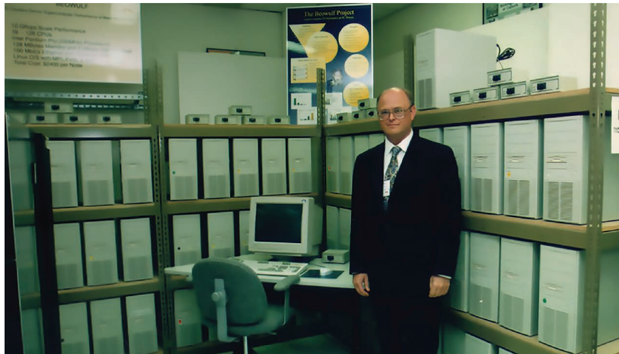
Thomas Sterling, who co-invented the Beowulf supercomputing cluster at Goddard Space Flight Center, poses with the Naegling cluster at California Technical Institute in 1997. Consisting of 120 Pentium Pro processors, Naegling was the first cluster to hit 10 gigaflops of sustained performance.
