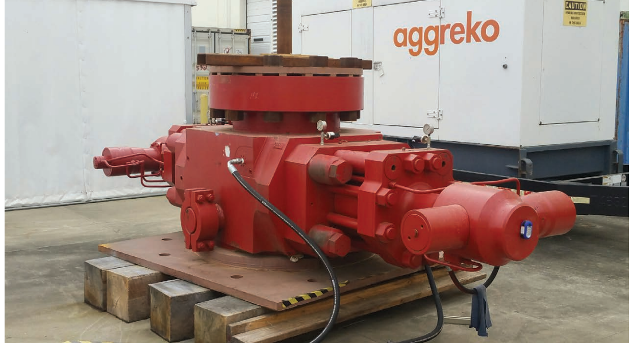
At demonstrations in late 2018 and early 2019, Bastion showed major players in the oil industry how five of its SureShear chambers (left) could power the very blowout preventer that failed to completely sever and seal the drill pipe in the Deepwater Horizon disaster (above). This 15,000-pound SureShear system replaces 170,000 pounds of compressed-gas tanks in a traditional system and severs the pipe about three times as fast.
