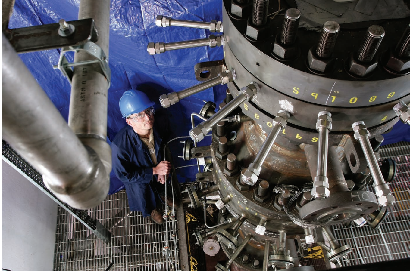
One alternative to burning coal is gasification, where coal is processed under high temperatures and pressures to extract synthetic gas and other products, which can then be used to generate electricity. GTI's R-Gas gasifier, shown here, helps relieve some of the environmental impact from the use of coal while also creating products for industry.
