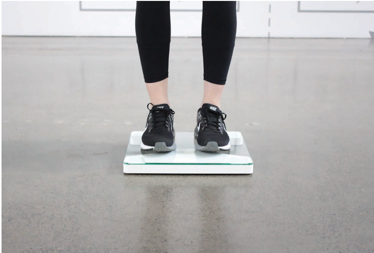
Based on a new technique pioneered in Johnson Space Center's Neurosciences Laboratory, the Zibrio balance scale assesses balance by applying algorithms to changes in pressure distribution over the course of a minute. The company found it could even predict a subject's likelihood of experiencing a fall.
