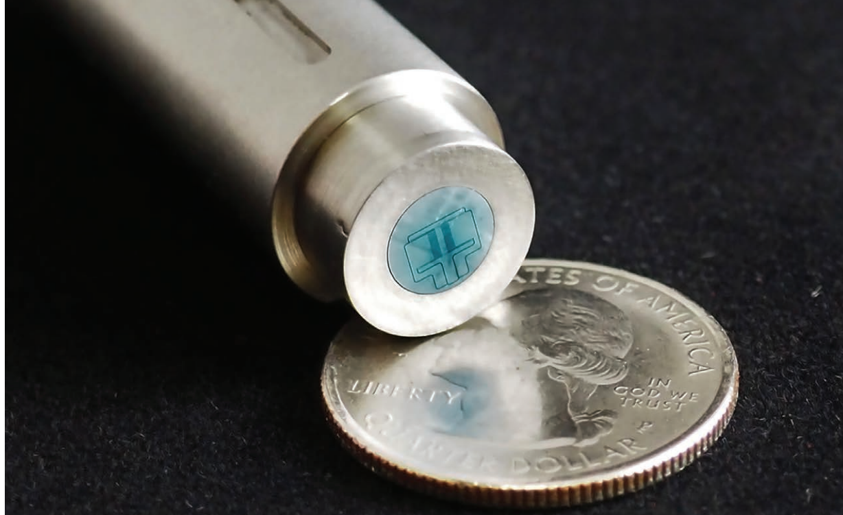
In IC's DirectShear sensors, a tiny, micromachined silicon sensor moves back and forth as air passes over it, changing the output voltage to indicate shear stress.
