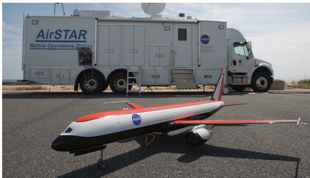
After developing its Algorithms for Uncertainty Representation and Analysis (AURA) software with Langley Research Center's help, Barron Associates tested and validated it on a fault-detection and control system for Langley's Generic Transport Model, part of the Center's Airborne Sub-Scale Transport Aircraft Research (AirSTAR) test bed.
