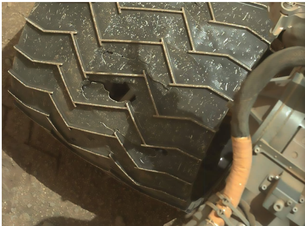
This image, taken by one of Curiosity's cameras in 2015, shows damage to the aluminum wheel from the rocky surface on Mars. In the future, Mars and lunar rovers may use a metallic glass coating over aluminum wheels—adding much-needed toughness without significantly increasing the overall weight.
