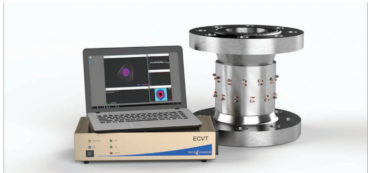
Tech4Imaging’s ECVT technology uses a series of capacitance plates surrounding a pipe to sense flows of up to three phases. A processor uses sophisticated mapping software to make sense of the data, calculating the flows and displaying three-dimensional images.
