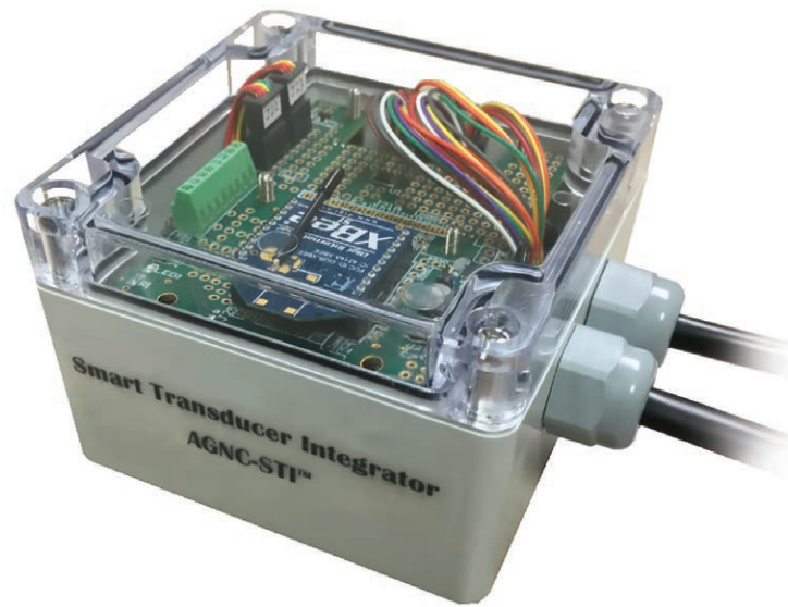
American GNC's work on smart sensor networks for Stennis led to the company's coremicro Reconfigurable Embedded Smart Sensor Node (left) and the Smart Transducer Integrator that can gather and package information from a sensor network (right).
