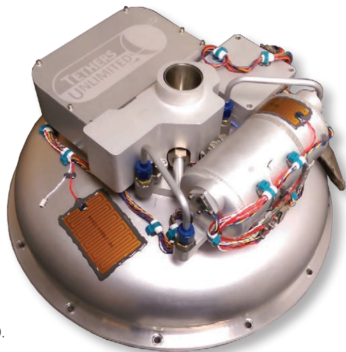
Tethers Unlimited's HYDROS-C thruster is intended to introduce propulsion capabilities to relatively tiny CubeSats, letting them maintain or change their orbits. It was slated to fly on NASA's Pathfinder Technology Demonstrator 1 in 2019.
