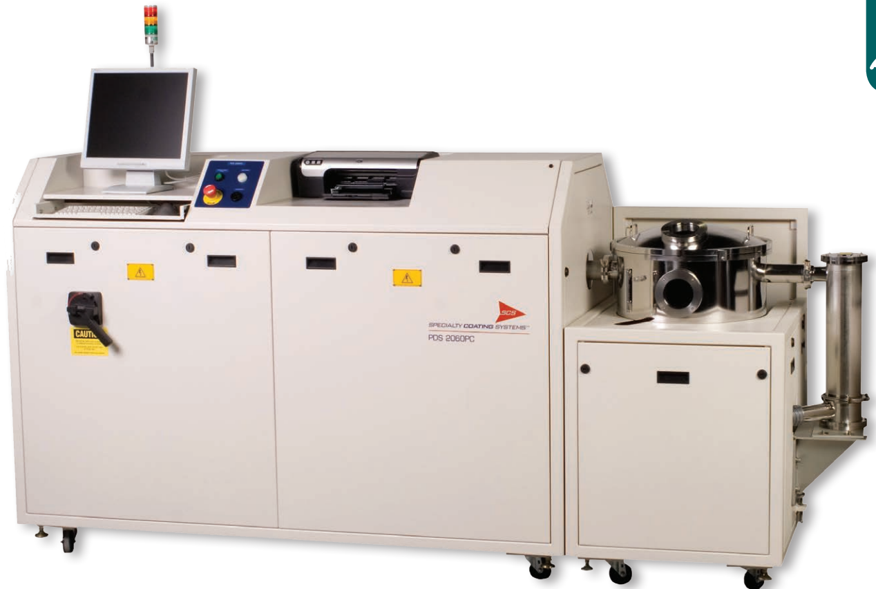
Applied in a vacuum with equipment like this device from Specialty Coating Systems Inc., Parylene coatings conform completely to the surfaces they cover.
