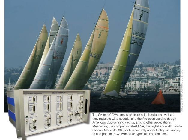
ranges that detect temperature and the higher temperatures that sense velocity. Conventional systems would instead use multiple sensors at different dedicated temperatures and risk burning out if temperatures are changed too rapidly.
