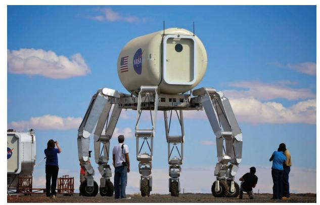
Much of the technology and expertise behind RoboSimian came from JPL's long history of building robots, such as the versatile, limbed and wheeled ATHLETE freight-carrying robots designed for planetary operations.
