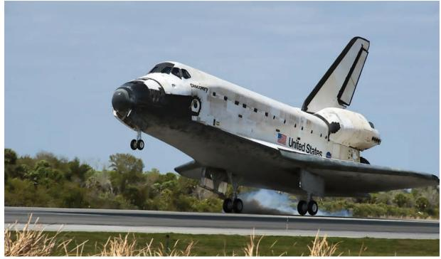
Proper tire pressure is crucial for a safe landing, but in the early days of the Space Shuttle Program, there was no good way to accurately gauge pressure in flight. Instead, engineers relied on extensive pre-flight ground tests to measure air loss over time.
