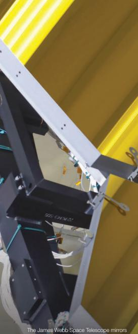
are removed from Marshall Space Flight Center's X-Ray and Cryogenic Facility following testing. The mirrors are made of beryllium in part because the material will deform predictably when taken from room temperature to near absolute zero. of light but sturdy mirrors NASA needed for Webb. After a Ebidding process, Materion won the contract to build the mirrors.
