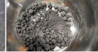
DSI customers can buy raw asteroid simulant powders or mixes of a range of grain sizes.
