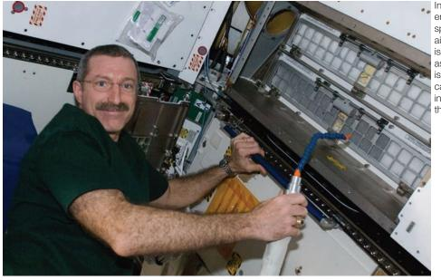
In a small, closed environment like the space station, keeping air clean and breathable is a serious chore. NASA astronaut Dan Burbank is shown here cleaning cabin air bacteria filters in the Tranquility node of the station in 2012.
