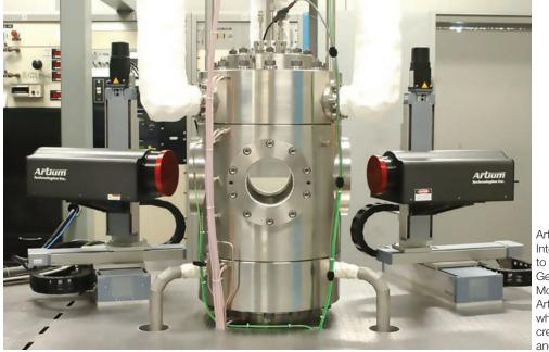
Artium's Phase Doppler Interferometer is used to test fuel injectors at a General Motors facility. Most automakers use Artium technology, which was originally created to test rocket and jet engines. by three different photodetectors. Bachalo first developed the method with the help of his partner at Aerometrics, Michael Houser.
