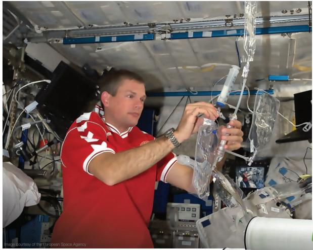
Astronauts on the ISS tested prototype water purification systems based on membranes infused with aquaporin proteins. The testing, which validated both forward and reverse osmosis-based systems, was sponsored by the European Space Agency and overseen by NASA.
