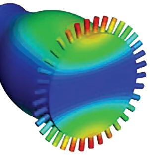
Gloyer-Taylor Laboratories (GTL) has created a software toolkit that models and analyzes structures for combustion instability, calculating the bulk flow of energy and then continuing on in layers, analyzing acoustics, vorticity, and then the thermal entropic energy. The company received multiple SBIR contracts from NASA to help design and test the toolkit, including the acoustics component called Resonance, which generated the image here.
