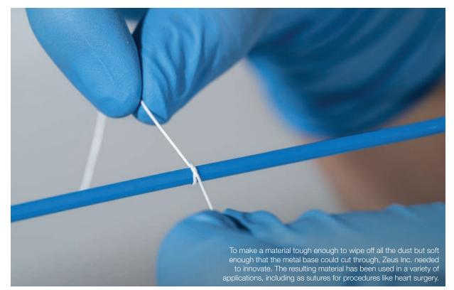
For many other applications, Black says, "the key to the material has always been that you're creating pores on the submicron level, which allows gas to move freely but not liquid." That makes it a great material for desiccant packaging aids—some of Zeus' customers use these when they ship sensitive electronics, for example.
