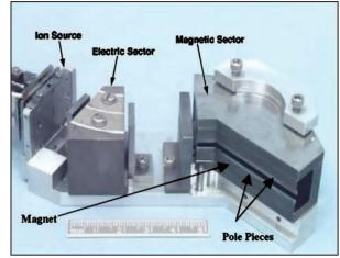
In the Mattauch-Herzog mass spectrometer configuration, ions are deflected first by an electrical field and then by a magnetic field to sort them by weight before they strike a focal plane that detects all the ions simultaneously. The CCD-based prototype created at JPL accomplished this within a small, rugged, inexpensive, energy-efficient device.
