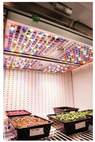
The Phytofy system's lighting capability and range of choice allow NASA researchers on Earth to simulate the lighting capabilities of the Advanced Plant Habitat, a growth chamber that astronauts began using on the ISS in early 2018.
