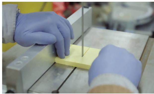
Aerogel Technologies, thanks to internal research and development as well as several technologies it has licensed from Glenn, manufacturers a class of aerogels it has branded Airloys. They can be made with a variety of properties, including high temperature tolerance, transparency, and varying degrees of flexibility and stiffness, and can be cut and machined into any shape.
