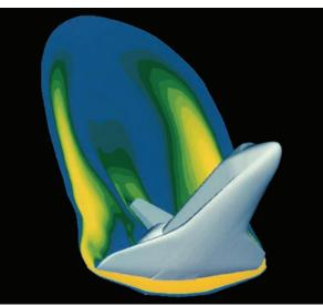
NASA uses a variety of tools to create simulations, including the computational fluid dynamics software used to simulate the aerodynamics of Space Shuttle descent here. The Distributed Observer Network (DON) can read and display any of those simulations.
