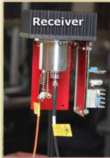
LaserMotive's success in the Power Beaming Challenge allowed the company to commercialize its Power over Fiber (PoF) technology, which provides electricity to devices through fiber optic cables. PoF is most commonly used to provide electricity to devices that require electrical or radio frequency isolation.
