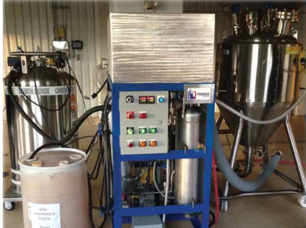
Pioneer Energy’s CO 2 Craft Brewery Recovery System can recapture about five tons of carbon dioxide per month, enough for a brewery that generates up to about 60,000 barrels per year, and units can be stacked to increase that capacity.
