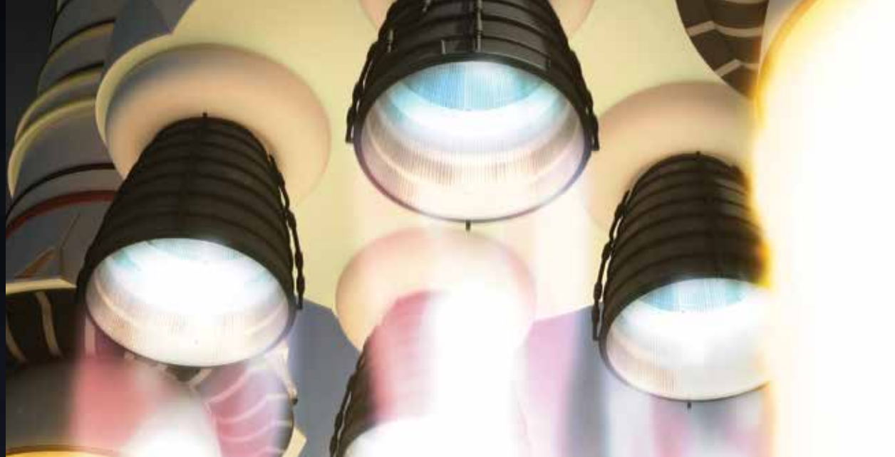
The Space Launch System's (SLS) core stage will be powered by the same RS-25 rocket engines that powered the Space Shuttle, although the SLS will use four engines rather than three, and they'll be optimized to increase thrust. Providing about 75 percent of the force at liftoff, though, will be solid-propellant boosters, again similar to those that launched the Shuttle, but bigger and more powerful. Altogether, the rocket will have 8.4 million pounds of thrust at liftoff.
