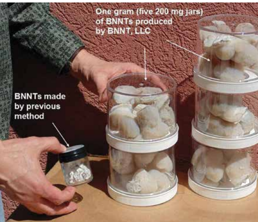
BNNT LLC has developed the technology to synthesize 200 milligrams of boron nitride nanotubes per hour. The company is making the material available to researchers who aim to take advantage of its molecular properties, such as its strength and heat resistance, for a variety of applications.
