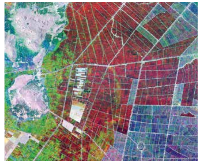
These two satellite images depict the An Giang Province in Vietnam's Mekong Delta, a major rice-producing region, at different times of year. Dark blue and black areas are inundated and have low biomass, while white and gray areas are other crops like row crops and trees. The differences in color indicate a change in the ratio between soil moisture and biomass.
