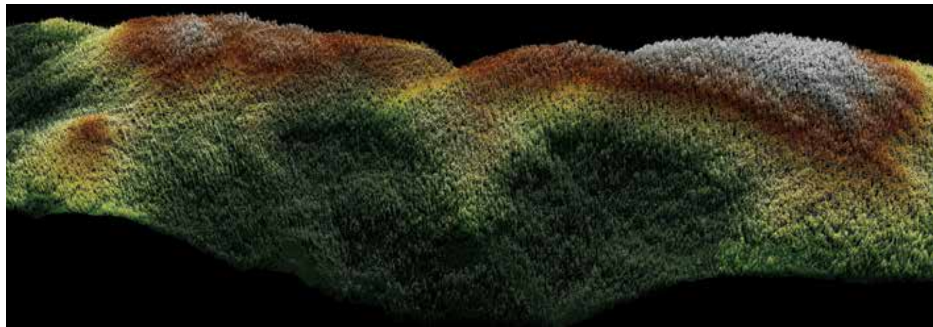
A Sigma imager captured this high-density lidar point cloud of a forested area in Sierra Nevada, California, in a single pass.
