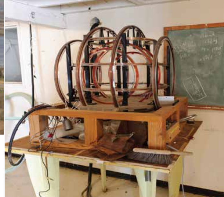
Helmholtz coils like this are used to manipulate magnetic fields. Two buildings at Ames Research Center helped test how Earth’s magnetic pull would interact with components of early spaceflight vehicles.
