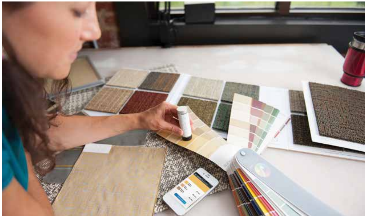
The NODE Chroma color sensors let the user upload a custom color set and reference colors against a library of hues.
