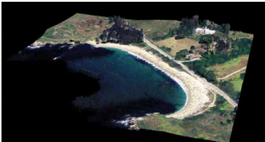
A lidar point cloud colored using simultaneously acquired photography by a Sigma Space imager shows the trees, grass, beach, and surf at Point Lobos in California. Meanwhile, a digital elevation model extracted from the data reveals the topography and bathymetry—that is, underwater elevations—of the same area, down to a sea depth of 13 meters.
