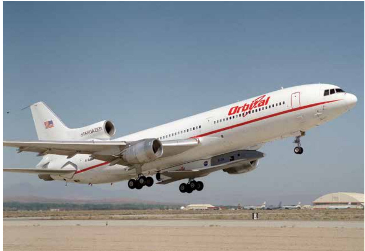
Orbital Sciences' modified L-1011 takes off with the NASA-funded X-34 Advanced Technology Demonstrator under its belly for the first captive-carry flight on June 29, 1999. Designed to launch from mid-air, the X-34 program was initiated by the Space Agency to test low-cost, reusable launch systems for putting payloads into space. Scientists at Ames Research Center developed Protective Ceramic Coating Material, or PCCM, to protect the spacecraft from the scorching heat of reentry into Earth's atmosphere.
