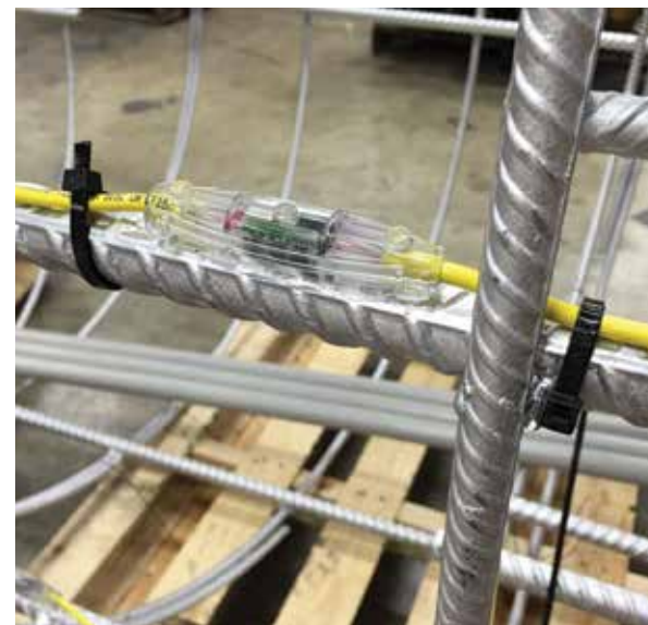
The thermal integrity profilers designed by Pile Dynamics Inc. are affixed to a rebar cage, which is then installed into a shaft and filled with cement. The profilers monitor the temperature of cement as it cures, which can alert engineers to any problems with the structural integrity of the cement before it dries.
