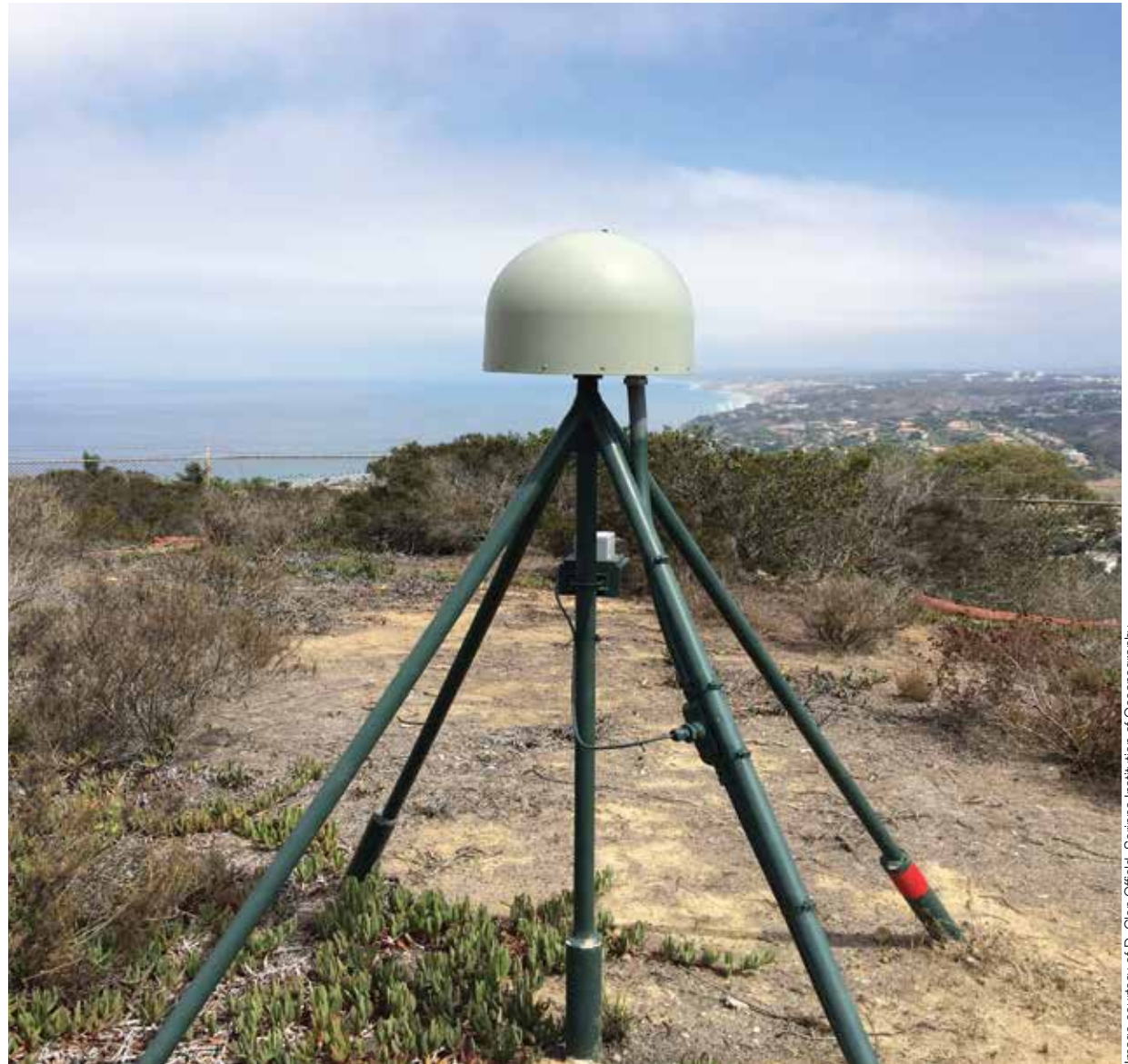
Thirty-seven GPS stations like this one on Mt. Soledad in San Diego have been added to the National Oceanic and Atmospheric Administration's meteorological GPS network in Southern California. Meanwhile, the Scripps Institution of Oceanography is outfitting the stations with accelerometers to enable early warning of earthquakes.
