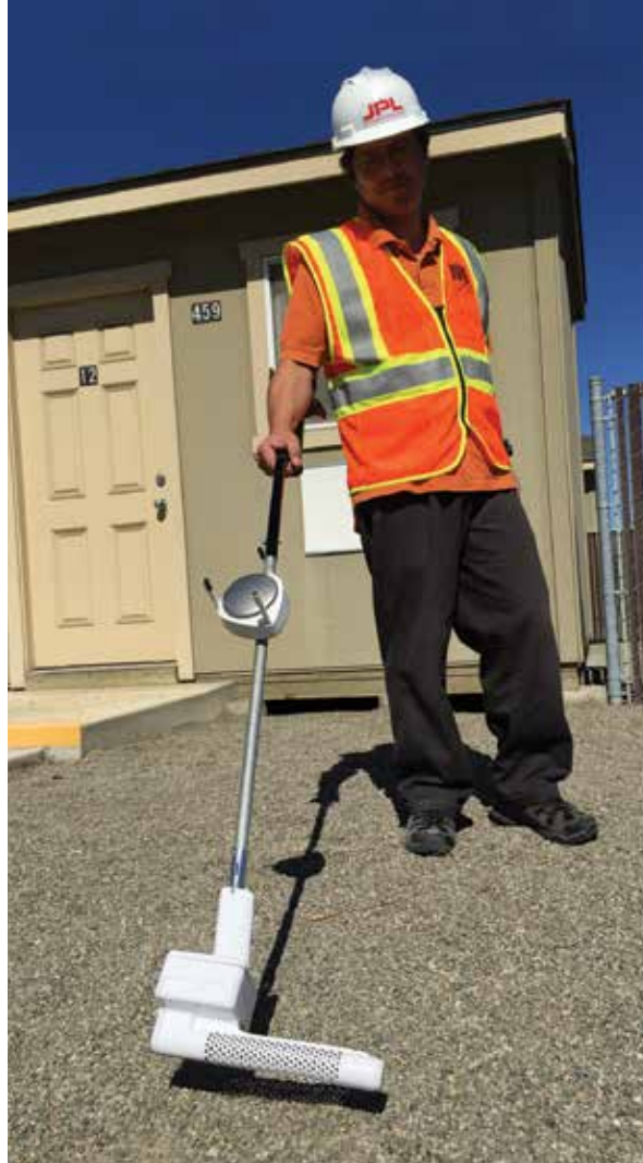
JPL senior scientist Lance Christensen tests the methane sensor he invented. Utility companies will use the device to detect gas pipe leaks, which are potentially dangerous and contribute to global warming.
