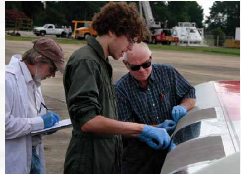
Researchers at NASA's Langley Research Center check results following preliminary NASA flight tests of nonstick coatings, which were selected in the hopes they could keep bug splatter off wings.
