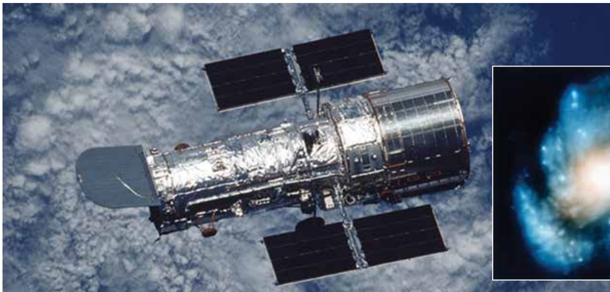
A misshapen mirror aboard the Hubble Space Telescope caused the first images beamed back to Earth to be fuzzy and out of focus. After the installation of new optics, tested by an aberrated beam analyzer invented by AOA Xinetics to ensure the new lenses would work perfectly, Hubble began sending back crystal-clear, vivid images from across the observable universe.
