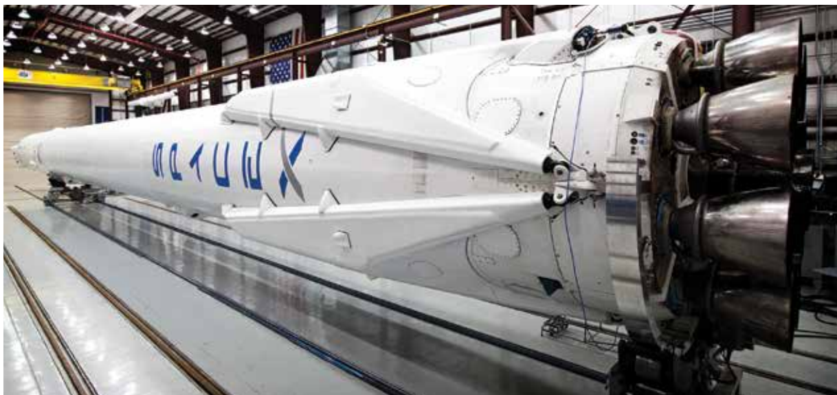
NASA ushered in an era of simpler, more efficient turbopumps with the invention of Fastrac in the 1990s. To minimize costly test stand launches, the Agency created the Generalized Fluid System Simulation Program, or GFSSP, to analyze computational fluid dynamics. SpaceX used Fastrac as a blueprint for developing its Merlin family of rocket engines for the Falcon 9 launch vehicle, which is responsible for delivering payloads to the ISS.
