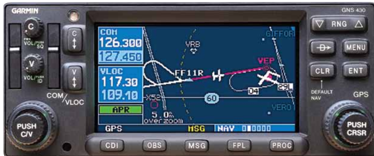
With help from a NASA contract, VoiceFlight Systems LLC developed a speech recognition interface for Garmin GPS units (like the one shown here). The interface enables general aviation pilots to enter destination points through speech rather than by hand.
