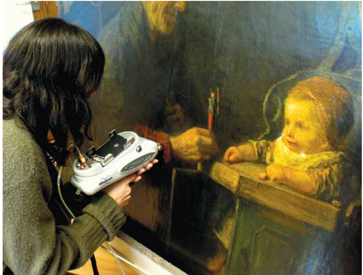
Bruker AXS’s XRF scanners quickly and easily identify the elements of an object down to parts-per-million—sufficient to analyze NASA spacecraft components or authenticate works of art.
