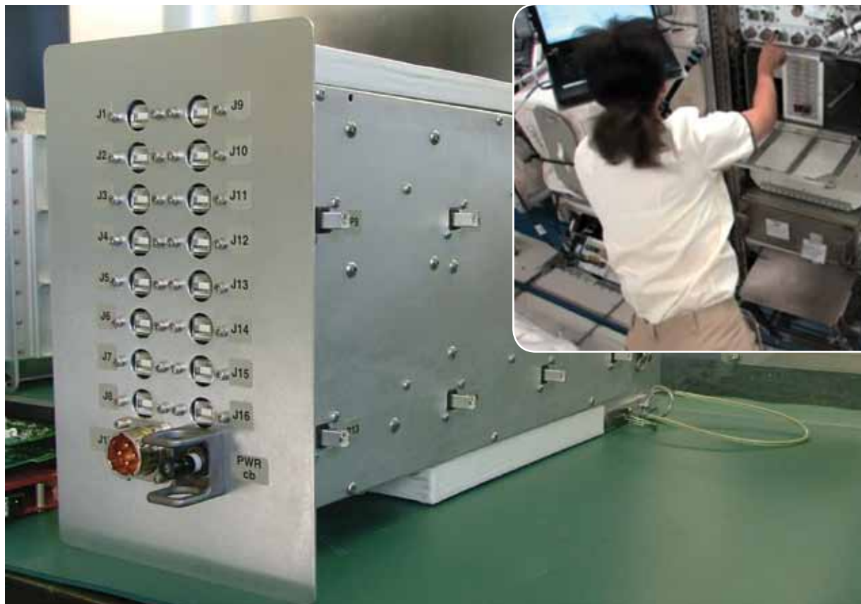
The NanoRacks Platform-1, seen in the inset image during installation on the International Space Station (ISS), can host up to 16 NanoLabs, which simply attach to plugs along the right and left sides of the platform. The “plug and play,” standardized system reduces the cost and increases the efficiency of space research.
