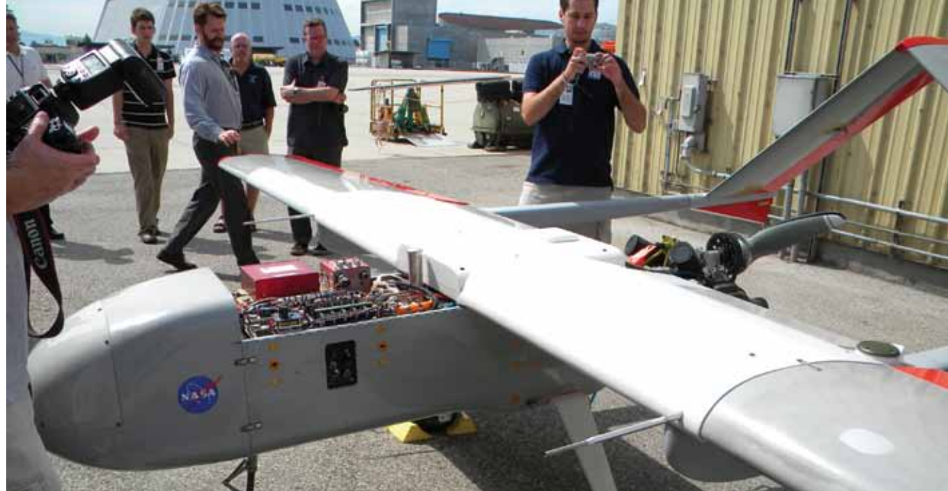
NASA’s SIERRA aircraft carried aloft sensors to measure greenhouse gasses and winds as part of a collaborative study that promises to provide important data for climate change and astrobiology research.
