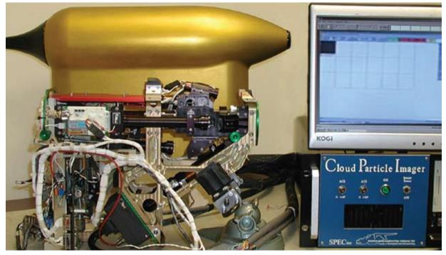
After SPEC's externally mounted CPI captures a particle's image, the system transmits the information to a computer and SPEC's CPI software, which crops and compresses the images. The system then stores the images and information for further analysis.
