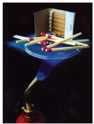
The remarkable insulating properties of aerogels have made them the focus of significant NASA research.
