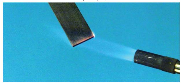
Dr. Ruth Pater of Langley Research Center developed RP-46, a polyimide resin capable of withstanding the high temperatures of aerospace applications.
