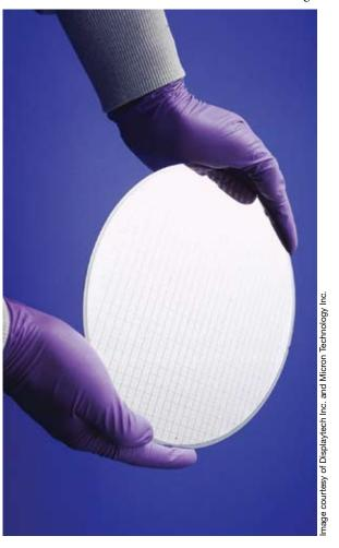
Ferroelectric liquid-crystal-on-silicon (FLCOS) panels need a smooth and shiny wafer top surface, which is possible with chemical mechanical planarization (CMP), a special technique of polishing semiconductor wafers to allow more metal layers—and smoother integrated-circuit surfaces.
