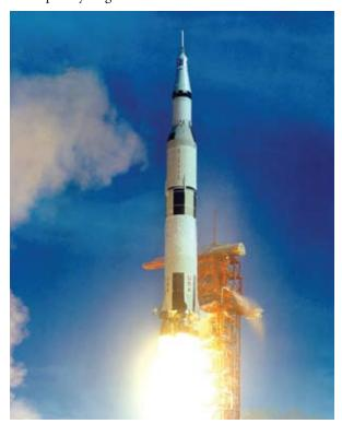
The Saturn V was a liquid-fueled expendable rocket used for Apollo and Skylab missions. Apollo 15, shown here, used over three-quarters of a million gallons of liquid oxygen and liquid hydrogen.
