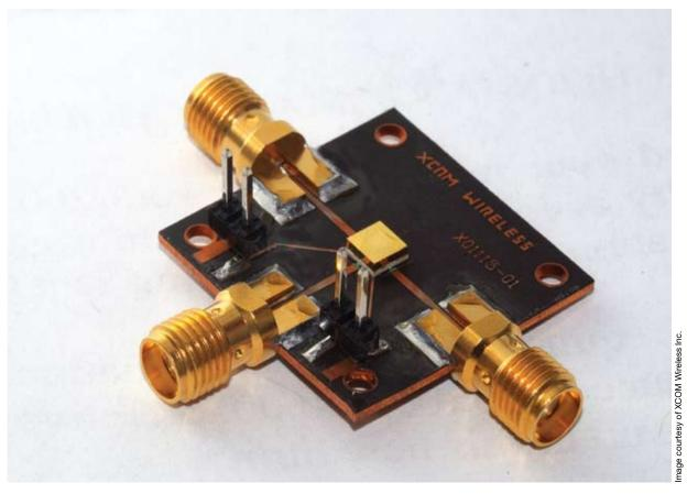
The XCOM Wireless XW3100 microelectromechanical single pole double throw relay, mounted on a radio frequency test coupon. According to the company, the XW3100 relays offer faster performance for automated test equipment, with frequency switching as high as 20 gigahertz.
