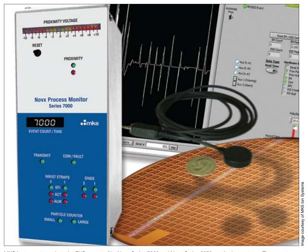
MKS Instruments markets the RVS as part of its Novx Series 7000 and Novx Series 3370 monitoring systems. These systems allow the customer to set the instrument sensitivity, thus tailoring the instrument's output to a specific need.
