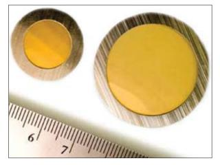
Lake Shore's SBIR-developed IR filters are ideal for astronomy applications, as well as for technologies like terahertz imaging.
