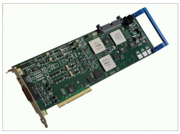
The TarsusPCM board—enhanced through Ulyssix's partnership with NASA—translates raw telemetry data into understandable measurements for engineer analysis, playing an essential role in satellite launch and ground support, as well as the testing of remote-controlled drones and jet engines.
