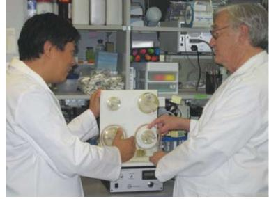
Regenetech scientists examine the company's bioreactors. Licensed from NASA, the bioreactor technology allows for rapid, healthy cell growth, providing for a quicker, cheaper source of adult stem cells for therapy and medical research.
