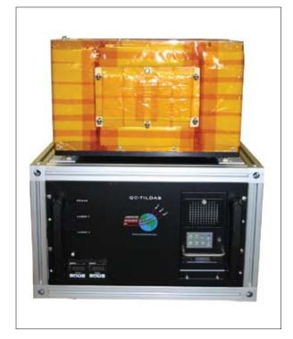
In 2002, ARI introduced a line of thermoelectrically cooled quantum cascade (QC) TILDAS instruments for use in its mobile laboratories. The QC-TILDAS instruments are incorporated into a system that contains the tunable laser, infrared detectors, power electronics, a microcomputer with integrated control and data analysis software, and an astigmatic multiple pass absorption cell.
