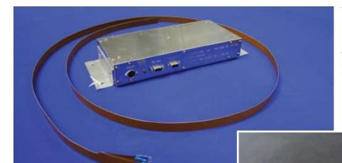
The Cryo-Tracker probe (at left) can monitor mass, levels, temperature, and pressure of stored cryogenic liquids. Below, the Cryo-Tracker probe descends into a large tank where a worker checks conditions.
