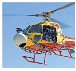
The flash lidar technology mounted on the nose of this helicopter may one day enable automated space docking and precise lunar landings.
