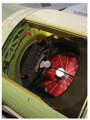
The infrared (IR) telescope of the Stratospheric Observatory for Infrared Astronomy (SOFIA) peers through the opening in the fuselage of its Boeing 747 mothership.
