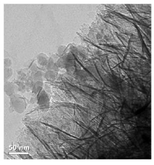
The NanoCeram water filter's nanoalumina fibers are shown here capturing fumed silica particles of a similar size to
