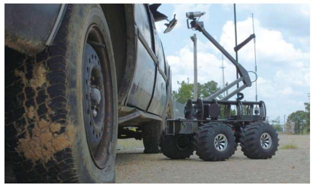
The MARCbot received multiple upgrades from engineers at NASA's Marshall Space Flight Center, and hundreds have now been deployed by the U.S. military overseas to help soldiers identify improvised explosive devices.
