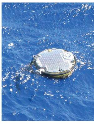
The satellite-communicating buoys designed by Airborne Technologies Inc. monitor ocean currents to locate areas where floating debris is likely to converge.
