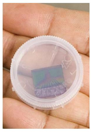
Containing millions of carbon nanotubes, the NASA biosensor can alert inspectors to minute amounts of potentially dangerous organic contaminants.
