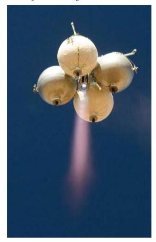
The Lunar Lander Challenge, one of the IPP's Centennial Challenges, involves building and flying a rocket-powered vehicle that simulates the flight of a vehicle on the Moon.
