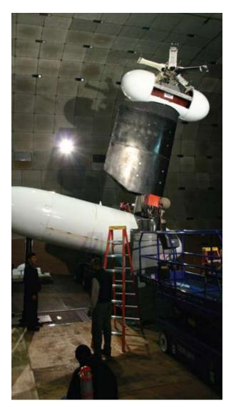
Engineers prepare the SMART rotor hub for wind tunnel testing. The rotor's piezoelectric enhancements help control noise and vibration.
