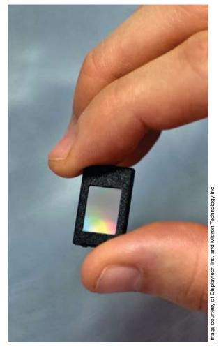
Displaytech Inc. uses its FLCOS technology to apply active matrix displays to a tiny silicon chip, with a final product smaller than a thumbnail. A thin layer of fast-switching liquid crystal material allows the circuitry to drive reflective pixels on the surface of the chip.
