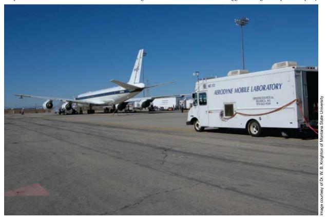
Aerodyne Research Inc. (ARI) uses its Tunable Infrared Laser Differential Absorption Spectrometer (TILDAS) instruments in its mobile laboratory to measure pollutant gasses and submicron particles in a DC-8's engine exhaust plumes.
