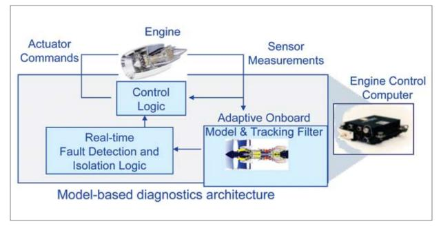
Sensor data fed into an aircraft's engine control computer can be used to constantly update an onboard adaptive engine model, which offers a continuous assessment of engine condition and performance, a key safety enhancement.
