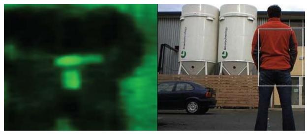
New security imaging products use the VDI diodes to detect passive terahertz waves, which can reveal images hidden behind common materials. The image on the left, returned from the security system, shows a gun hidden under the man's jacket.
